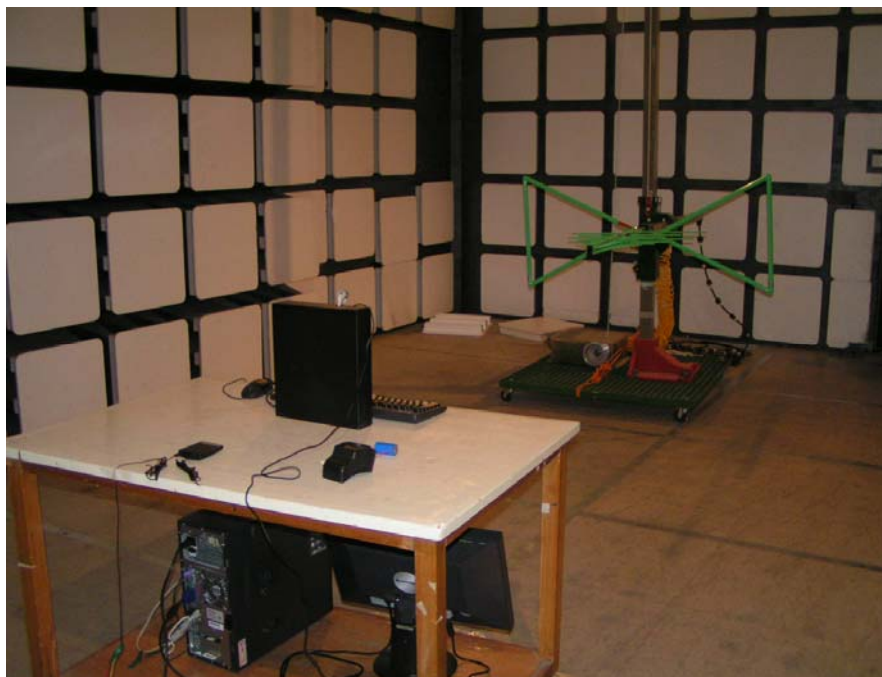
Field Strength Emissions Test Set-up (Below 1GHz)
