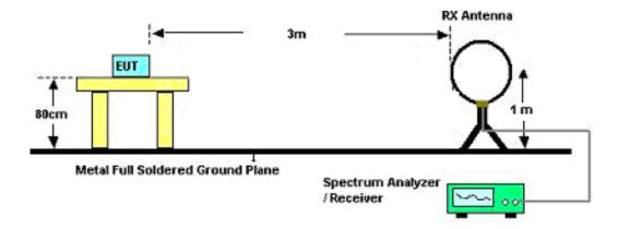
For Radiated Emissions: 30MHz~1GHz
