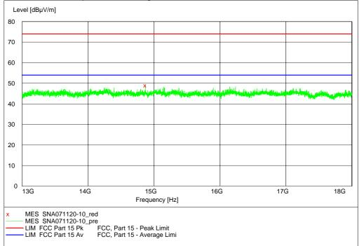
13 – 18 GHz, max peak and average at a distance of 3 m on the highest TX channel
