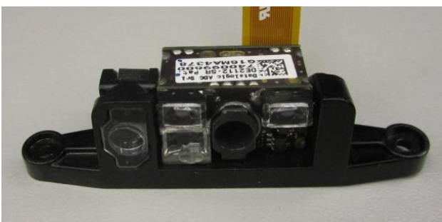
2D Imager with plastic support and Green Spot
