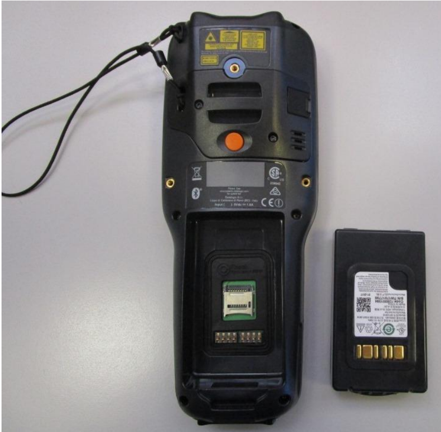
Rear View with battery disconnected
