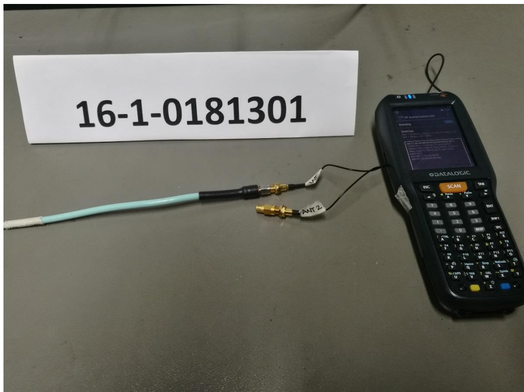
Photograph 2: Set Up 2-Close View- ANT1 Used + ANT2 Terminated with 50 \Omega [WLAN 5 GHz Modes]
