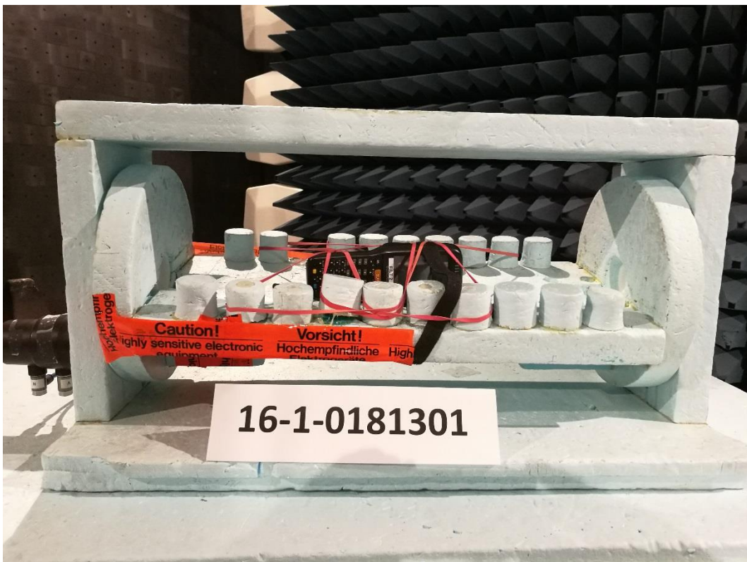
Photograph 12: Set Up 1-Close View - 30 MHz-1 GHz - EUT Laying 0°- Front Side
