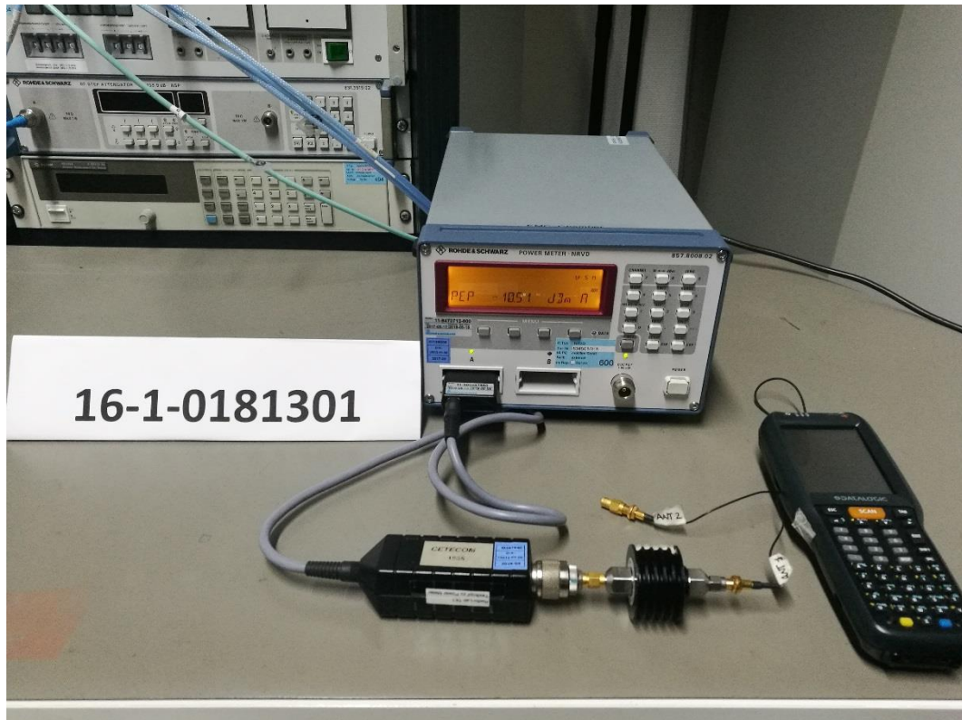
Photograph 3: Set Up 2-Overall View-ANT1 Used + ANT2 Terminated with 50 \Omega [WLAN 5 GHz Modes]
