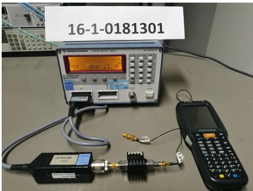
Photograph 4: Set Up 2-Close View-ANT1 Used + ANT2 Terminated with 50 \Omega [WLAN 5 GHz Modes]
