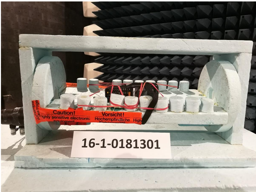
Photograph 10: Set Up 1-Close View - 30 MHz-1 GHz - EUT Laying 0° - Front Side
