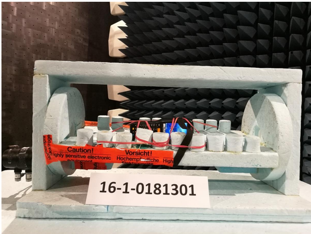
Photograph 6: Set Up 1-Close View -9 kHz-30 MHz- EUT Laying 0°- Front Side
