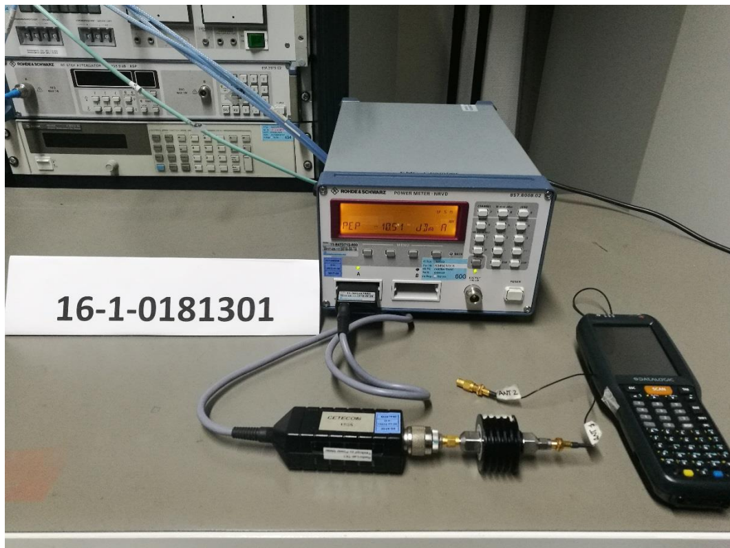
Photograph 1: Set Up 2-Overall View-ANT1 Used + ANT2 Terminated with 50 \Omega
