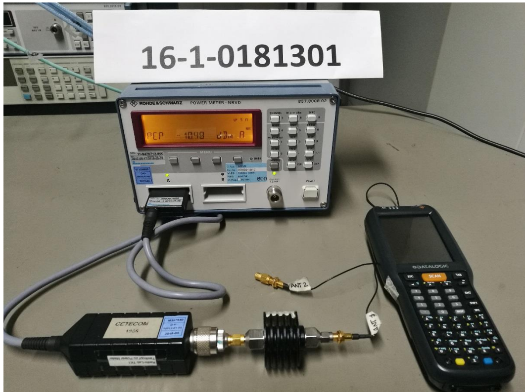
Photograph 5: Set Up 2-Close View-ANT1 Used + ANT2 Terminated with 50 \Omega [WLAN b/g Modes]
