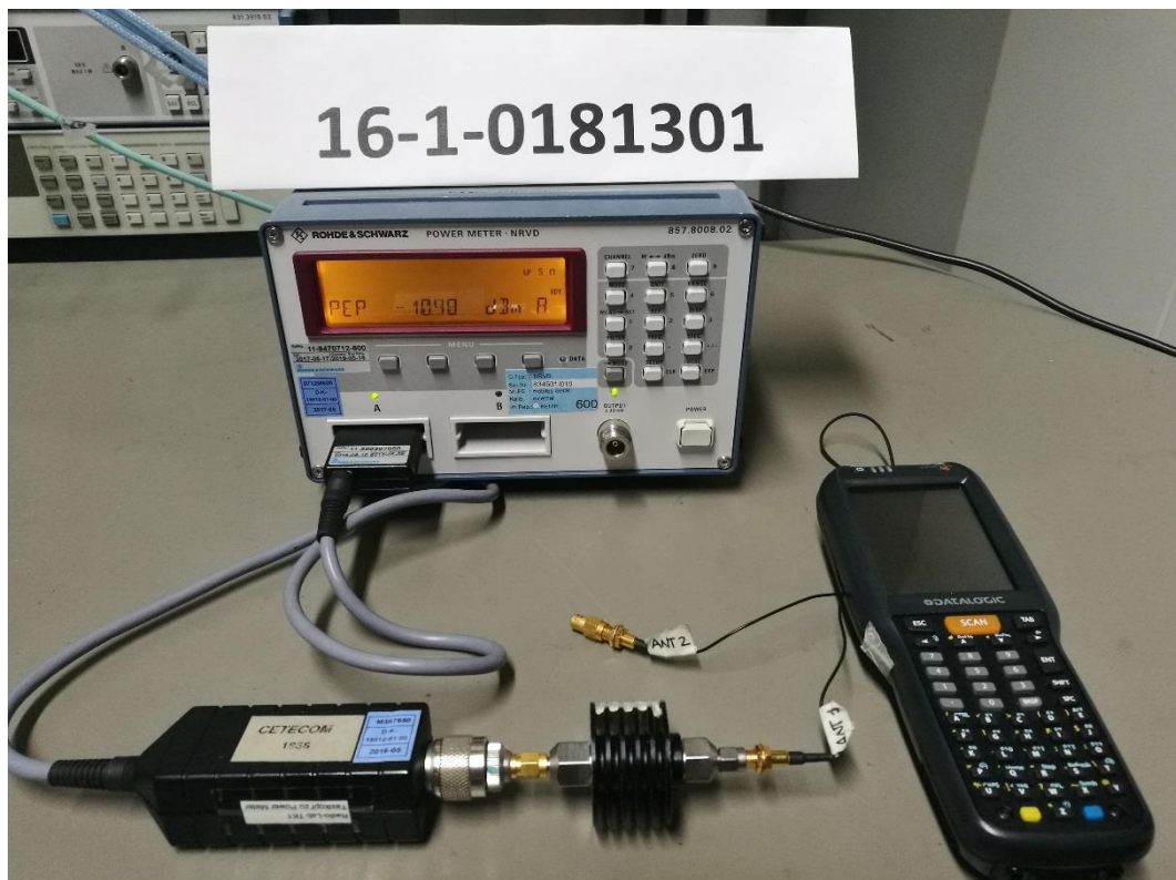
Photograph 6: Set Up 2-Close View-ANT1 Used + ANT2 Terminated with 50 \Omega [WLAN n Mode-MIMO]
