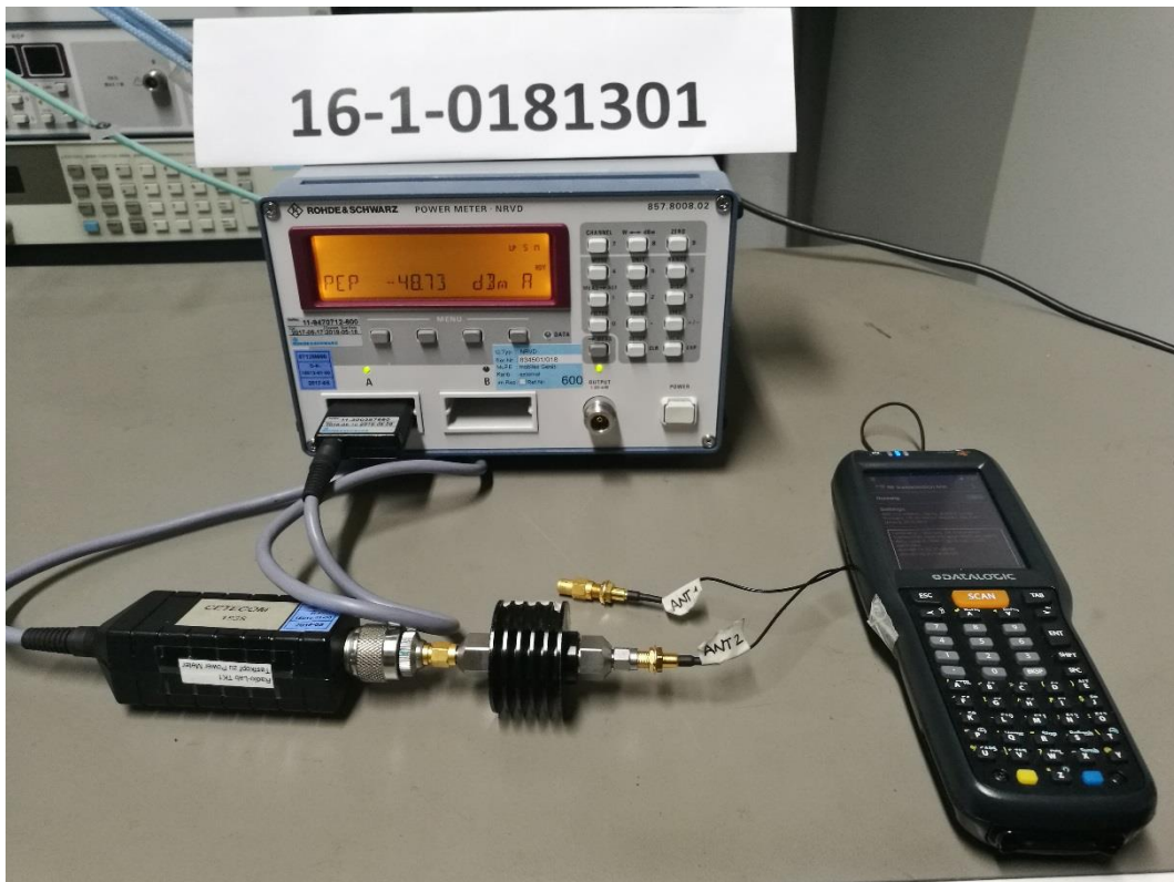
Photograph 7: Set Up 2-Close View-ANT2 Used + ANT1 Terminated with 50 \Omega [WLAN n Mode-MIMO]
