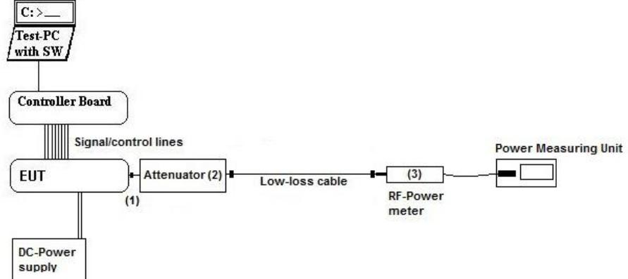
**Testing method:** ANSI C63.10:2013, KDB 558074 D01 DTS Meas.Guidance v04
