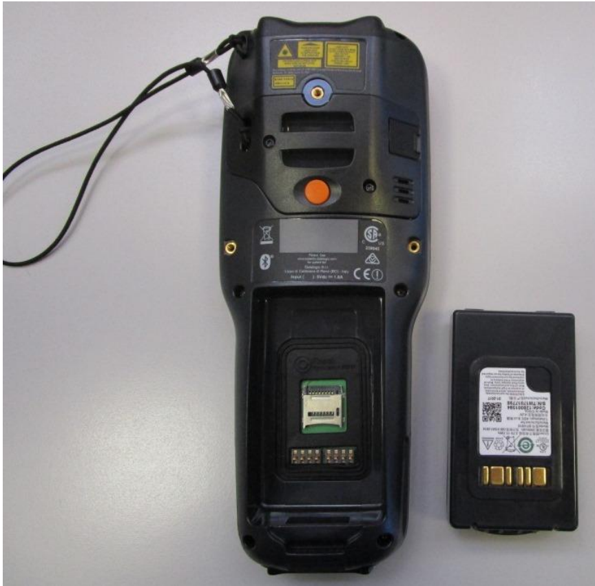
Photograph 5: SKORPIO X4 - Rear View with battery disconnected
