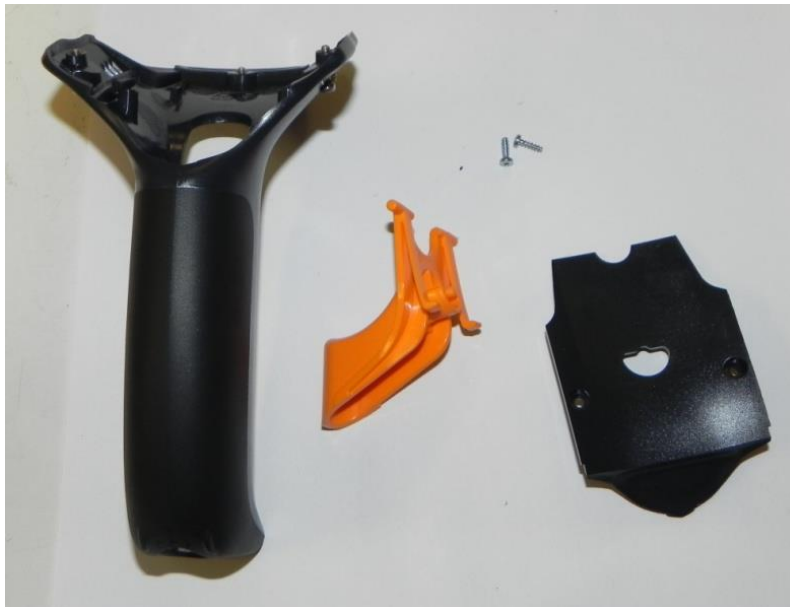
Photograph 6: SKORPIO X4 – Handle Assembly disconnected
