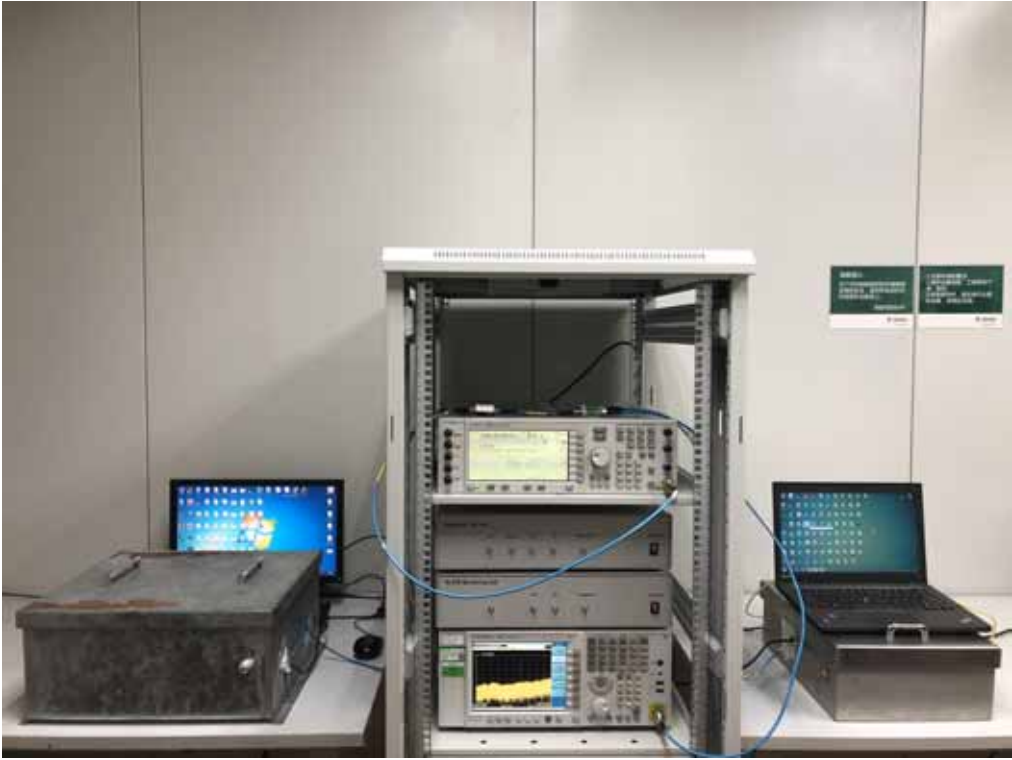
DFS Set-up Photo: Slave and Spectrum Analyzer
