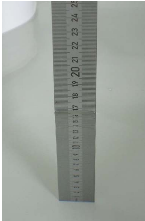
Fig. 12: Liquid depth for 2450 MHz body worn measurements.
