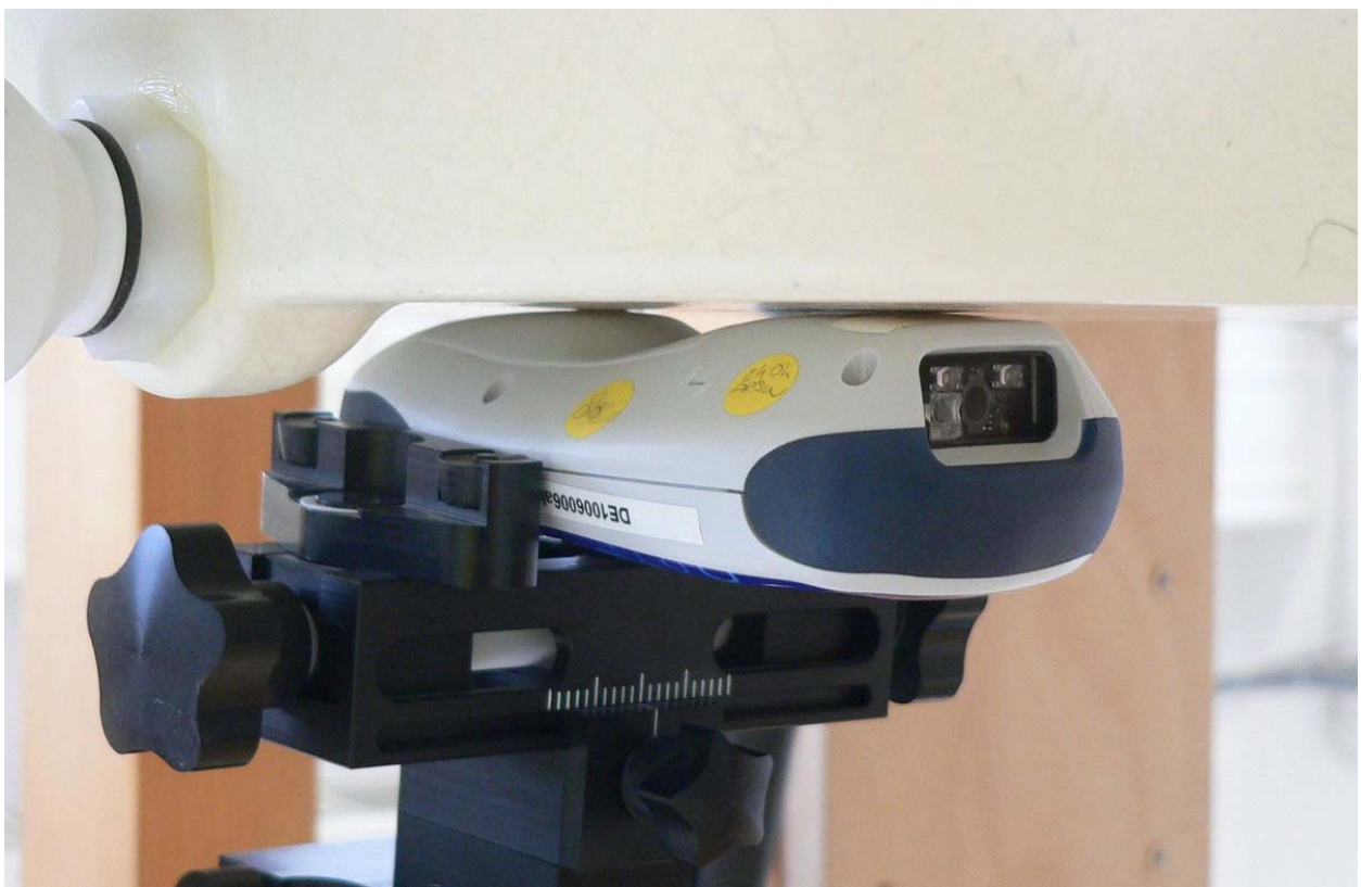
Fig. 9: Body worn configuration, position 2, back side towards the phantom.
