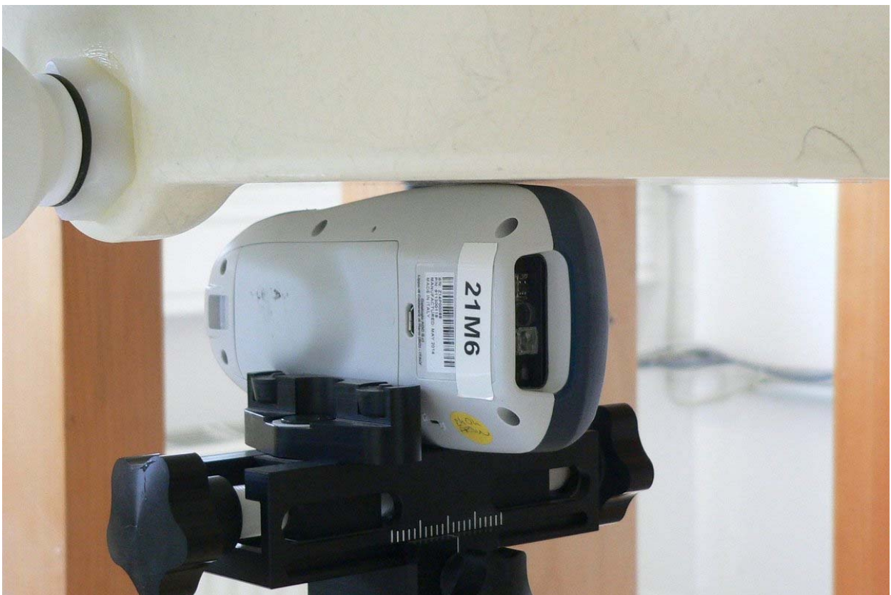
Fig. 11: Body worn configuration, position 4, right side towards the phantom.
