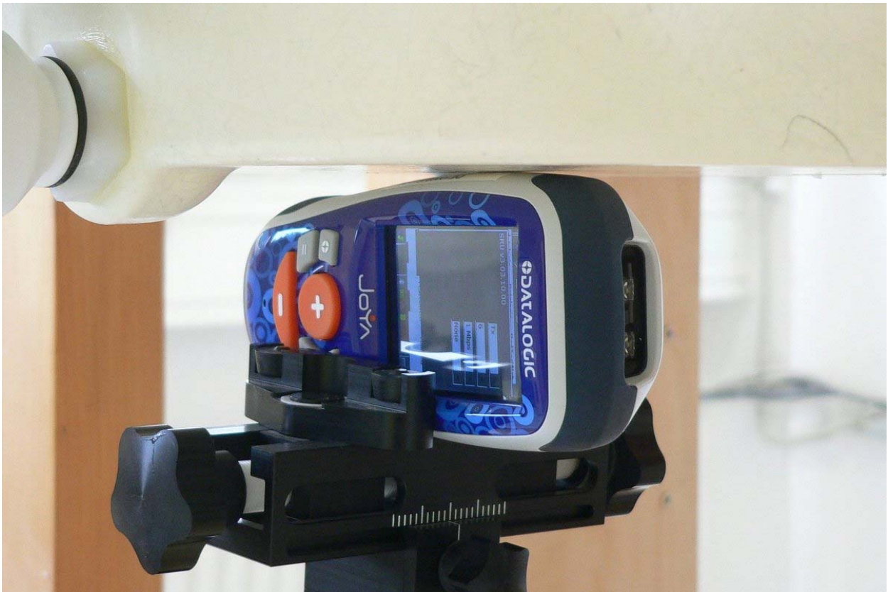
Fig. 10: Body worn configuration, position 3, left side towards the phantom.
