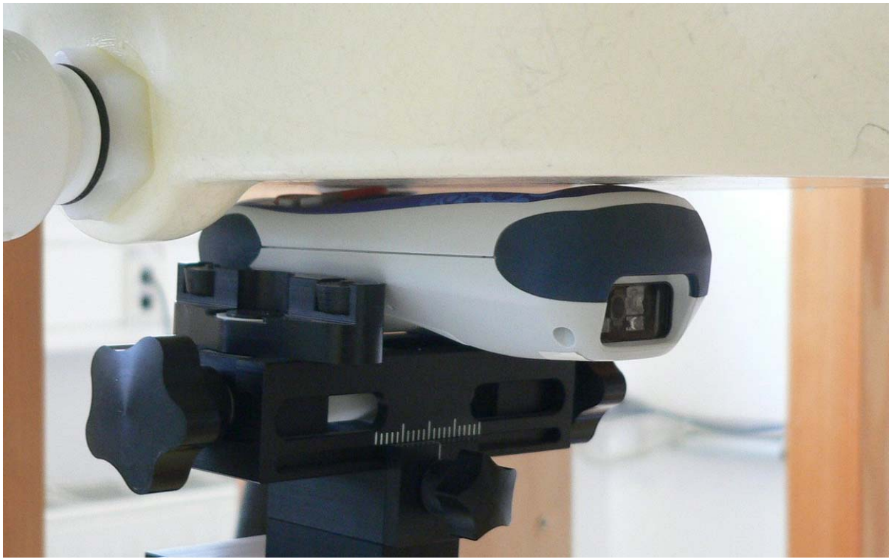
Fig. 8: Body worn configuration, position 1, front side towards the phantom.
