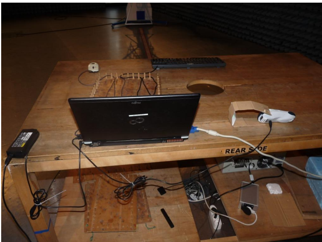
Photo 4: Test setup for radiated measurements, unintentional radiator §15) single device setup, computer peripheral.
