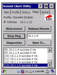
The *Diagnostic* button displays the radio configuration and dumps available profiles
