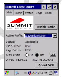
The *Active Profile* window displays the current profile and lets user to change it. The *Disable Radio* button turns off the radio card; after deactivation the same button changes to *Enable Radio* so the radio can be reactivated. To close the application, press the close button at upper-right corner of window.
