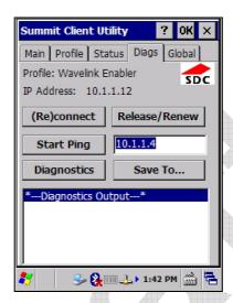
The (Re)connect button disables and re-connects radio card. The Release/Renew button releases and renews the radio interface IP address.
