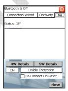
By tapping on the "HW Details" and "SW Details" buttons, information about the mobile computer Bluetooth® hardware and software will be displayed, while the "Enable Encryption" button starts encryption of the
