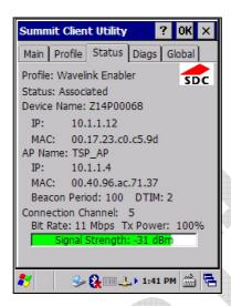
User can read current profile name, client device name, IP address and MAC address. The Access Point to which the terminal is currently associated t is specified by name, IP address and MAC address. User can also read the signal strength (dBm), the transmission power percentage, the WiFi channel, the rate (Mbps).
