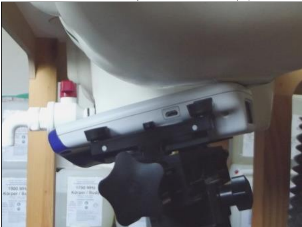
Photo 20: Measurement position – left hand tilted 15° (HH)
