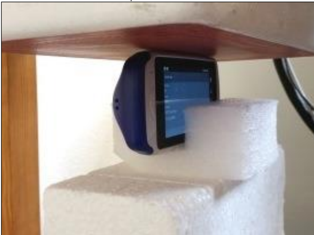
Photo 30: Measurement position - left side HH with 0mm distance
