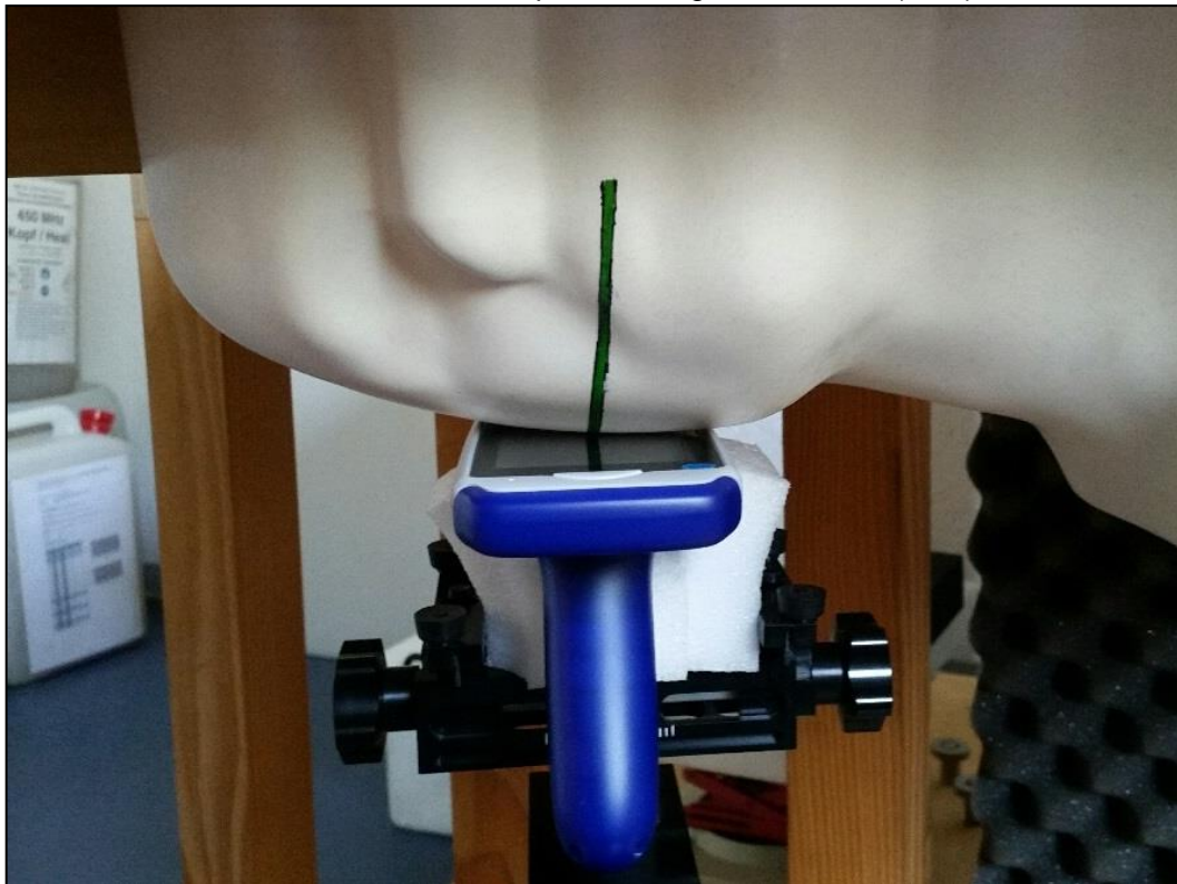
Photo 28: Measurement position - front side HH with 0mm distance
