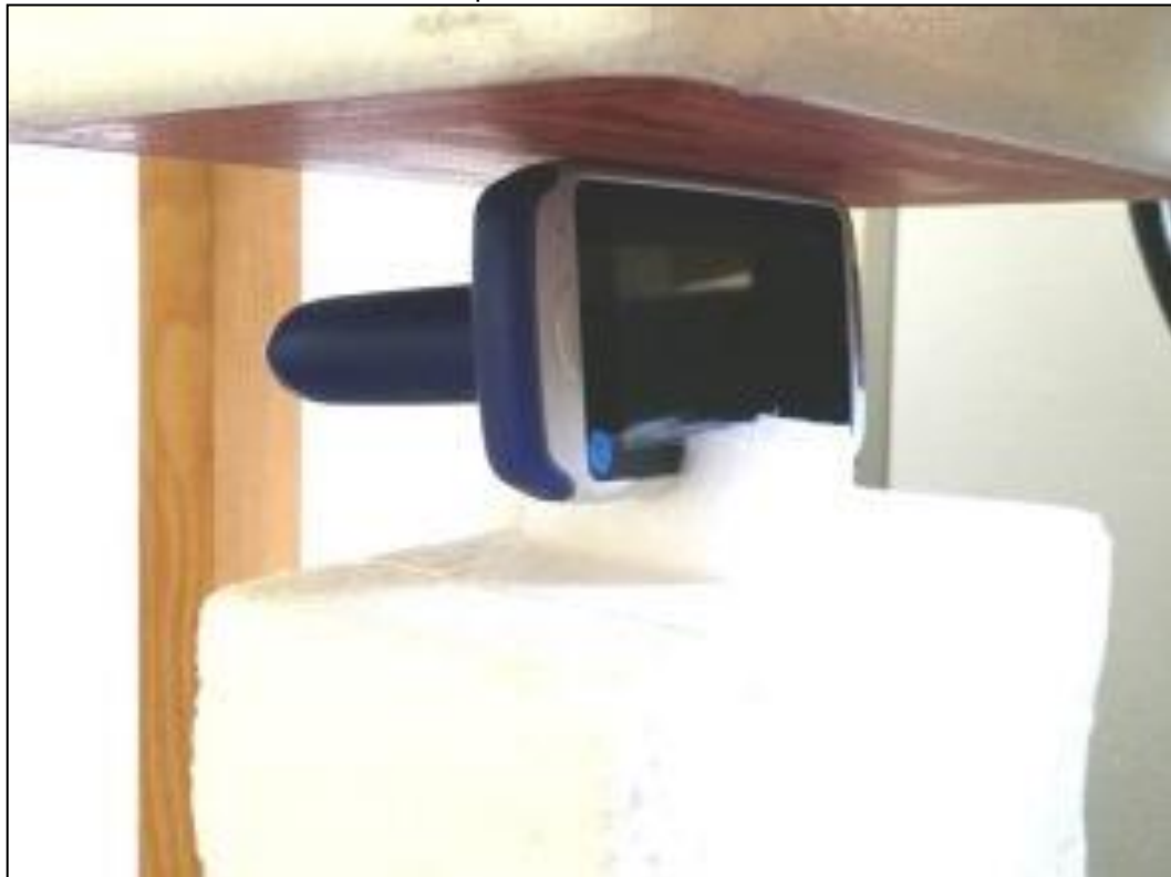
Photo 32: Measurement position - left side GUN with 0mm distance
