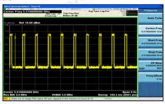
Duty Cycle: 17.98525 % \*The Channel Loading must over 17%
