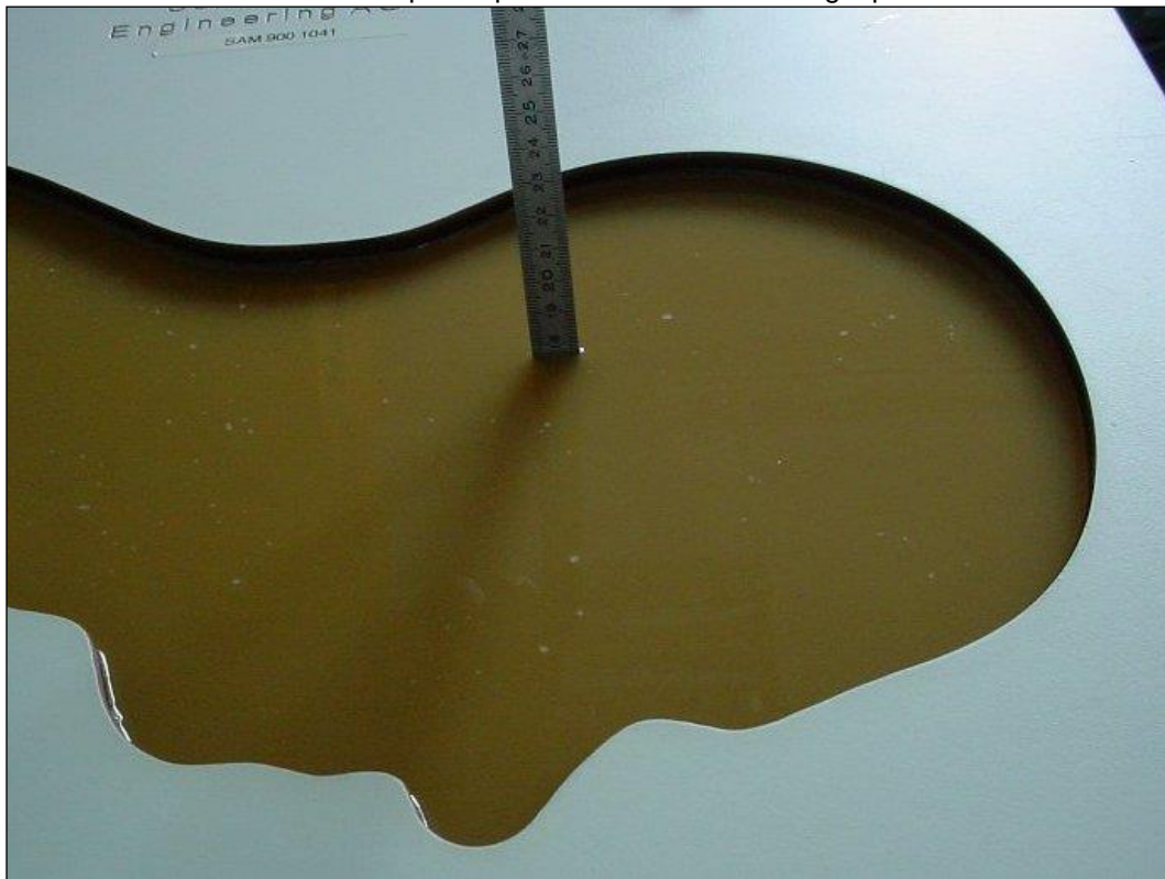
Photo 4: Liquid depth 5 GHz body simulating liquid
