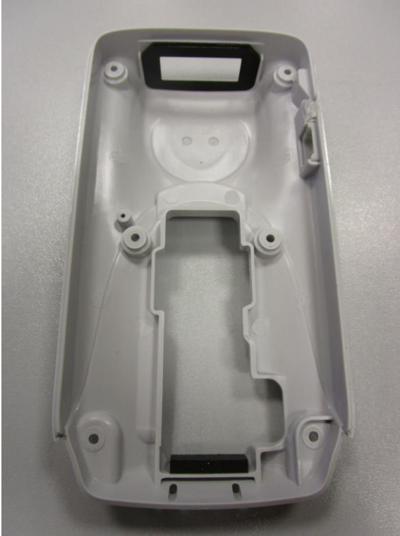
Bottom housing – Hand Held assembly
