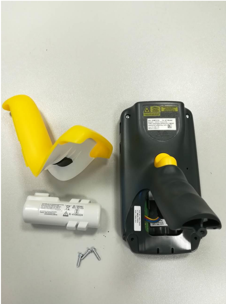
Rear View (battery housing opened) - Gun version
