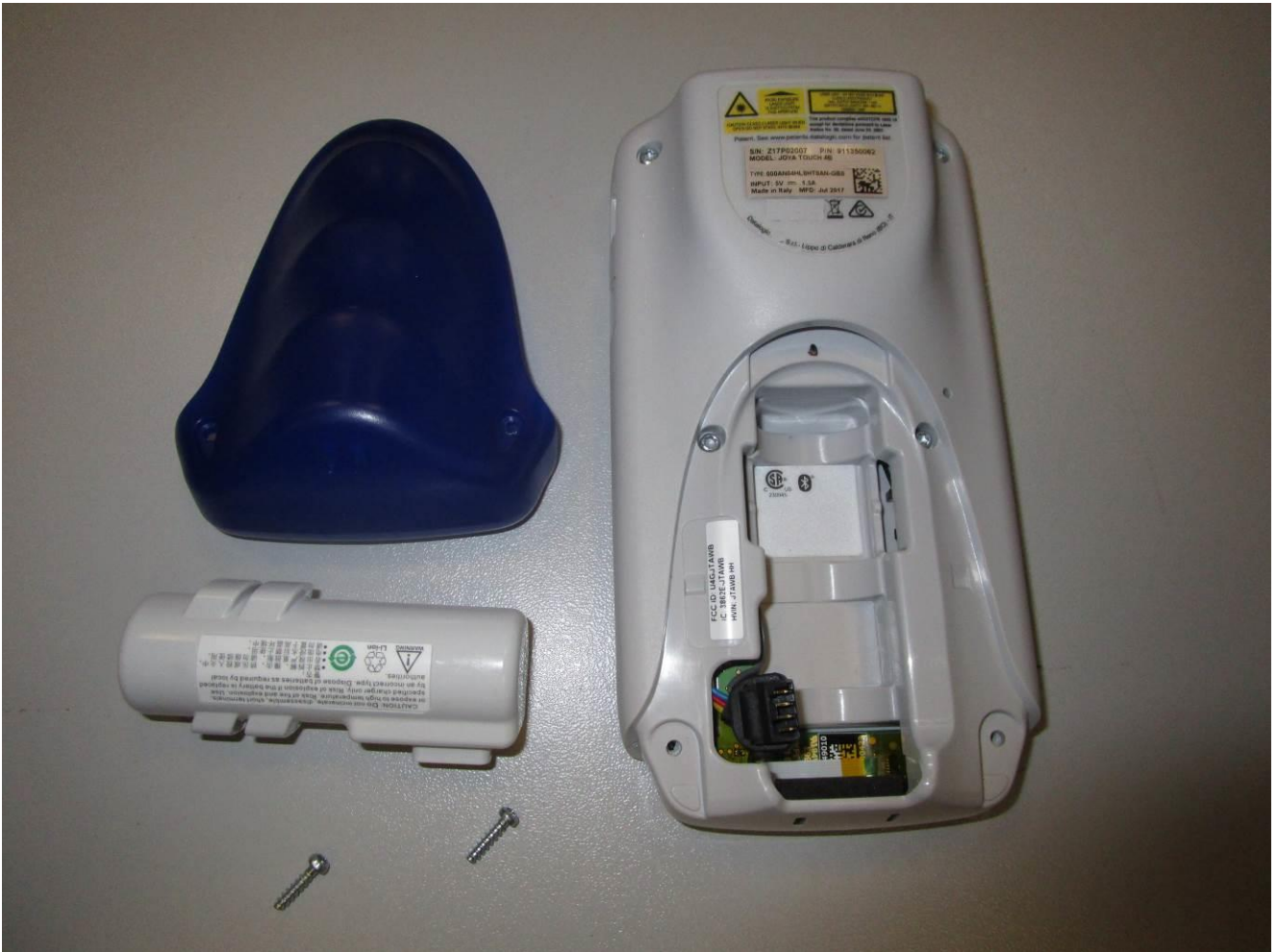
Rear View (battery housing opened) - Hand Held version
