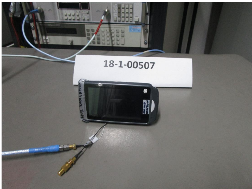
Photograph 1: Setup for conducted power (close view)
