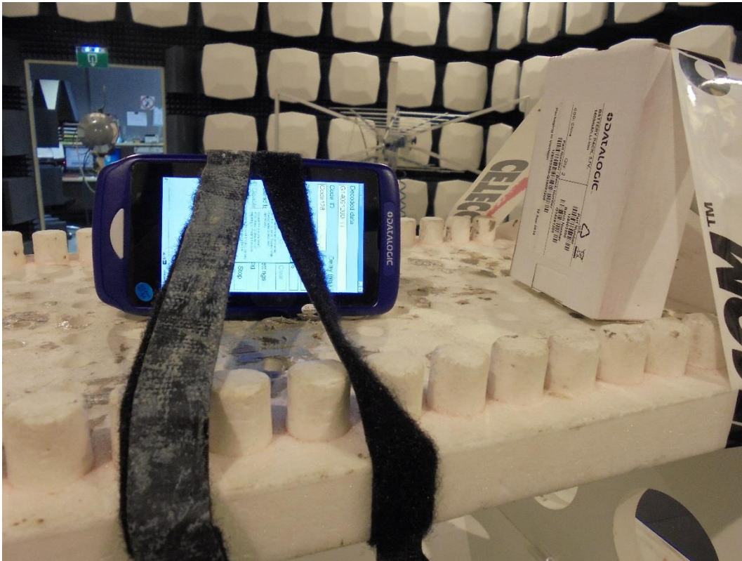
Photograph 8: Radiated measurement set-up (close up view_front side)_EUT 0°
