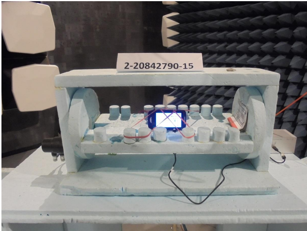
Photograph 4: Radiated measurement set-up (close up view_front side)_EUT 0°
