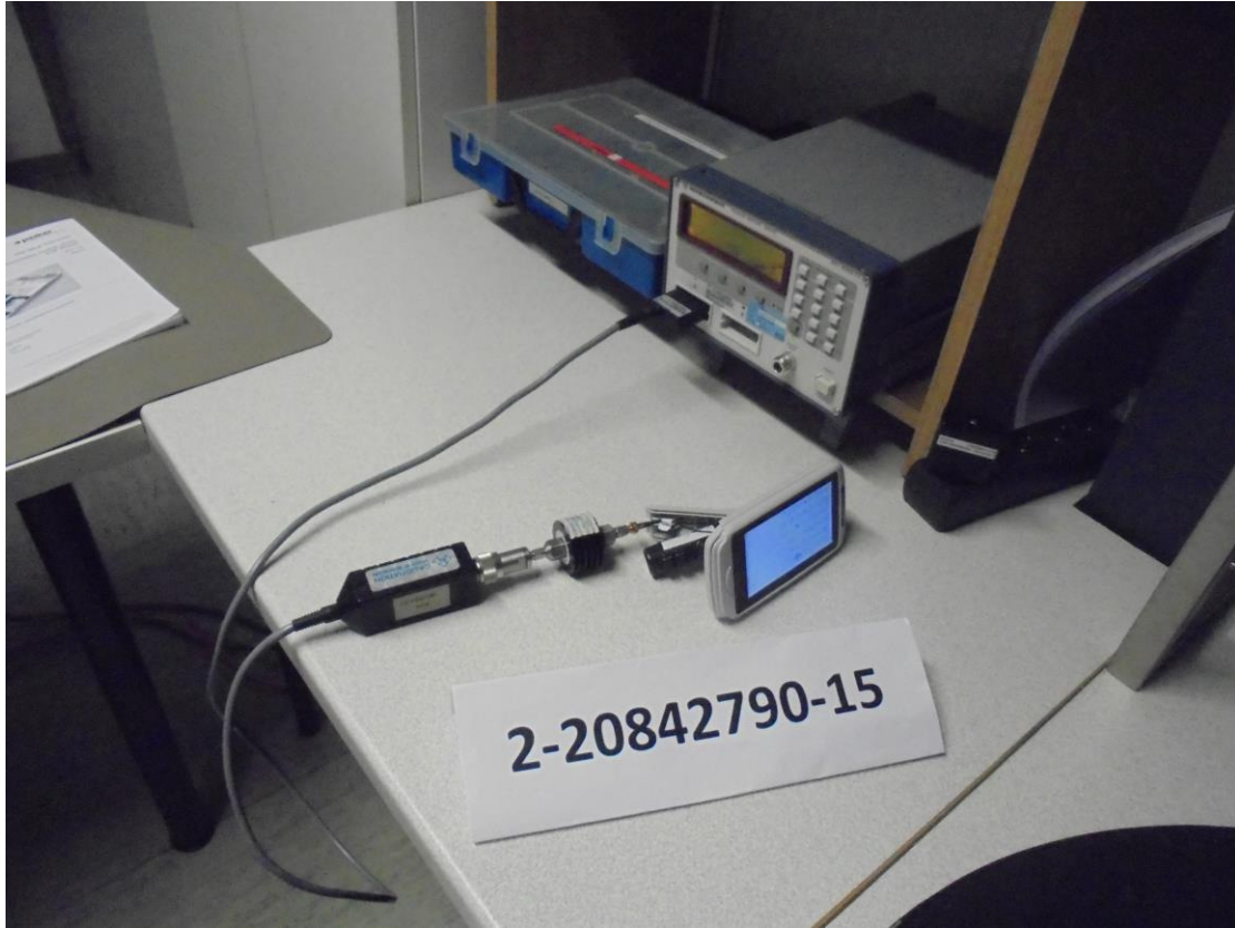
Photograph 3: Conducted measurement power meter set-up (overview_front side)
