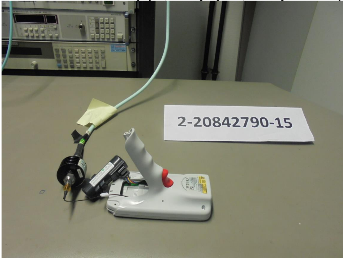
Photograph 1: Conducted measurement set-up (close up view_front side)
