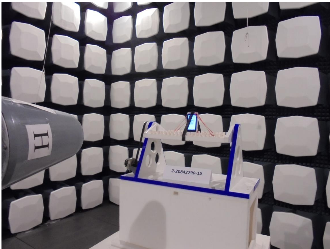
Photograph 16: Radiated measurement set-up (overview_front side) _EUT 0°
