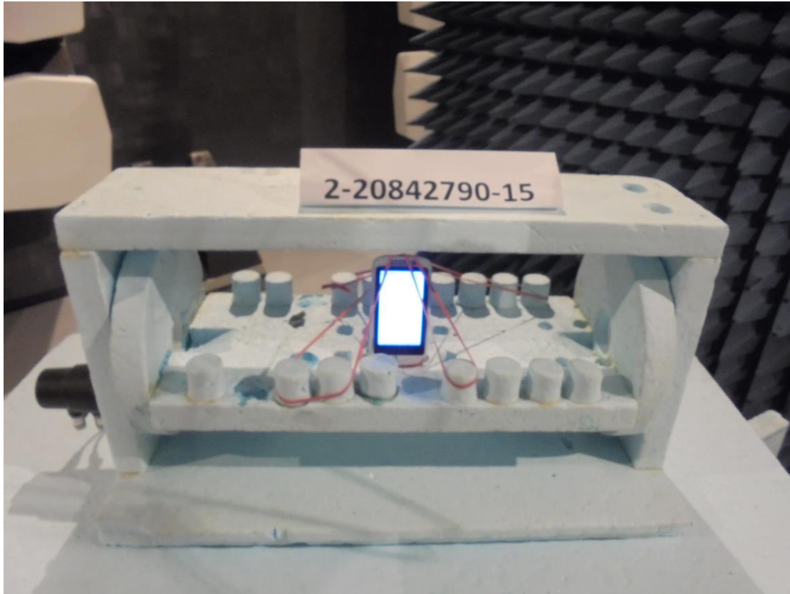
Photograph 10: Radiated measurement set-up (close up view_front side)_EUT 0°
