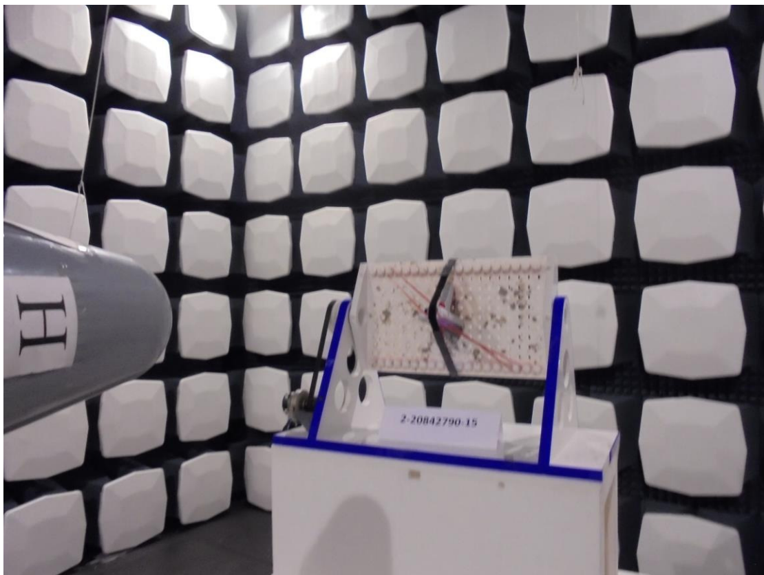
Photograph 17: Radiated measurement set-up (overview_front side) _EUT 90°
