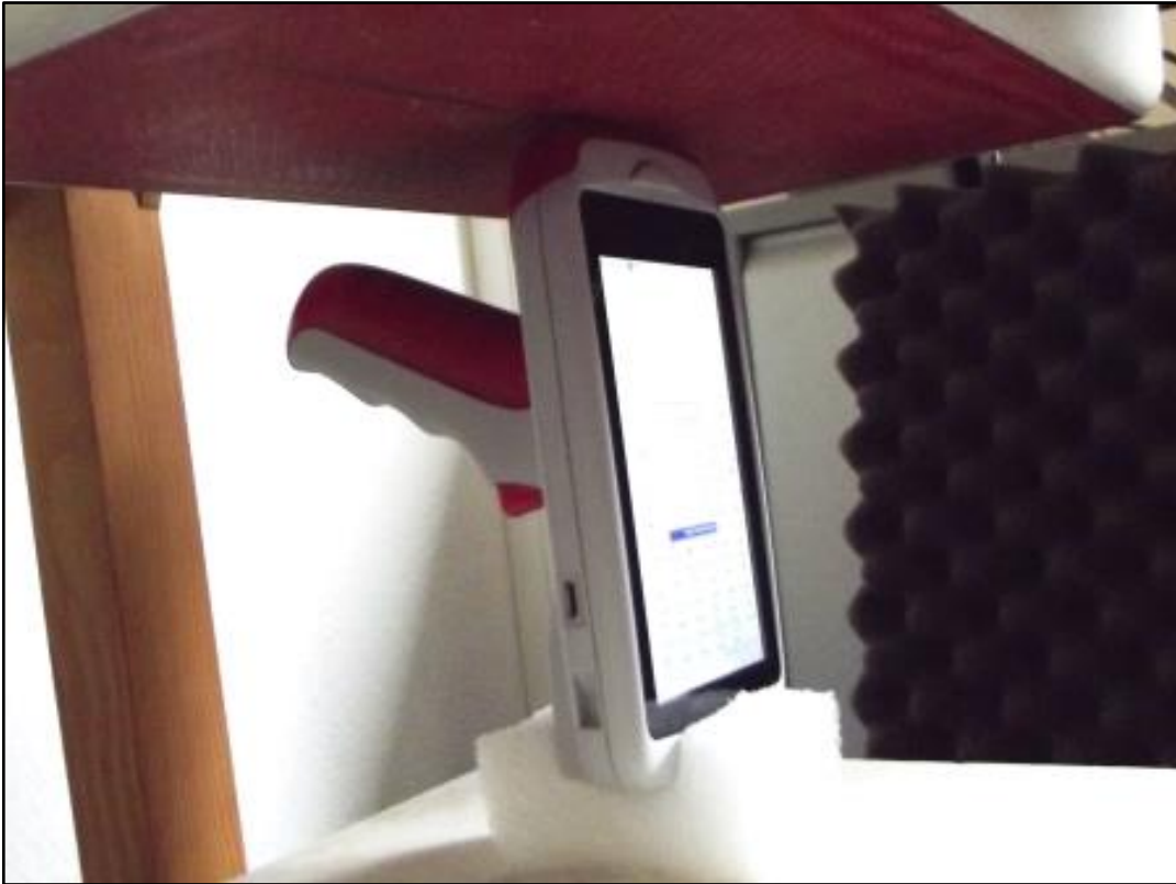
Photo 21: Test position bottom side with 0mm distance (Gun)
