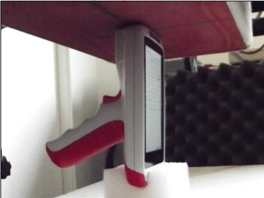
Photo 20: Test position top side with 0mm distance (Gun)
