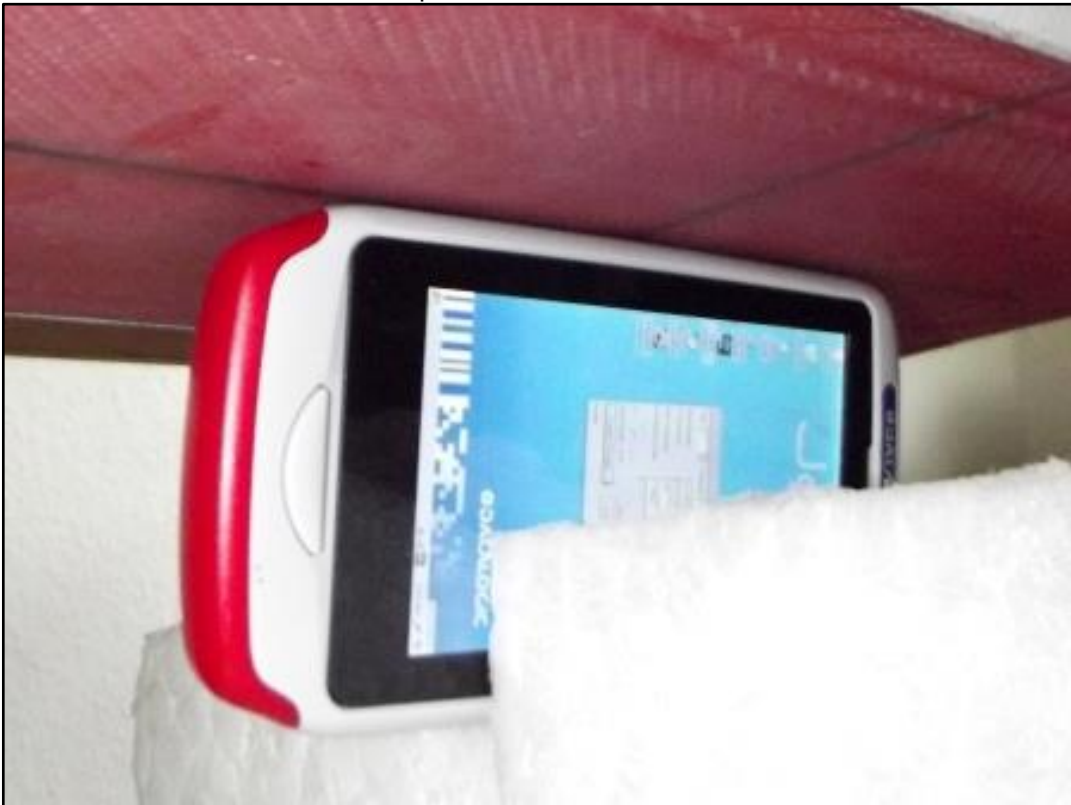
Photo 14: Test position left side with 0mm distance
