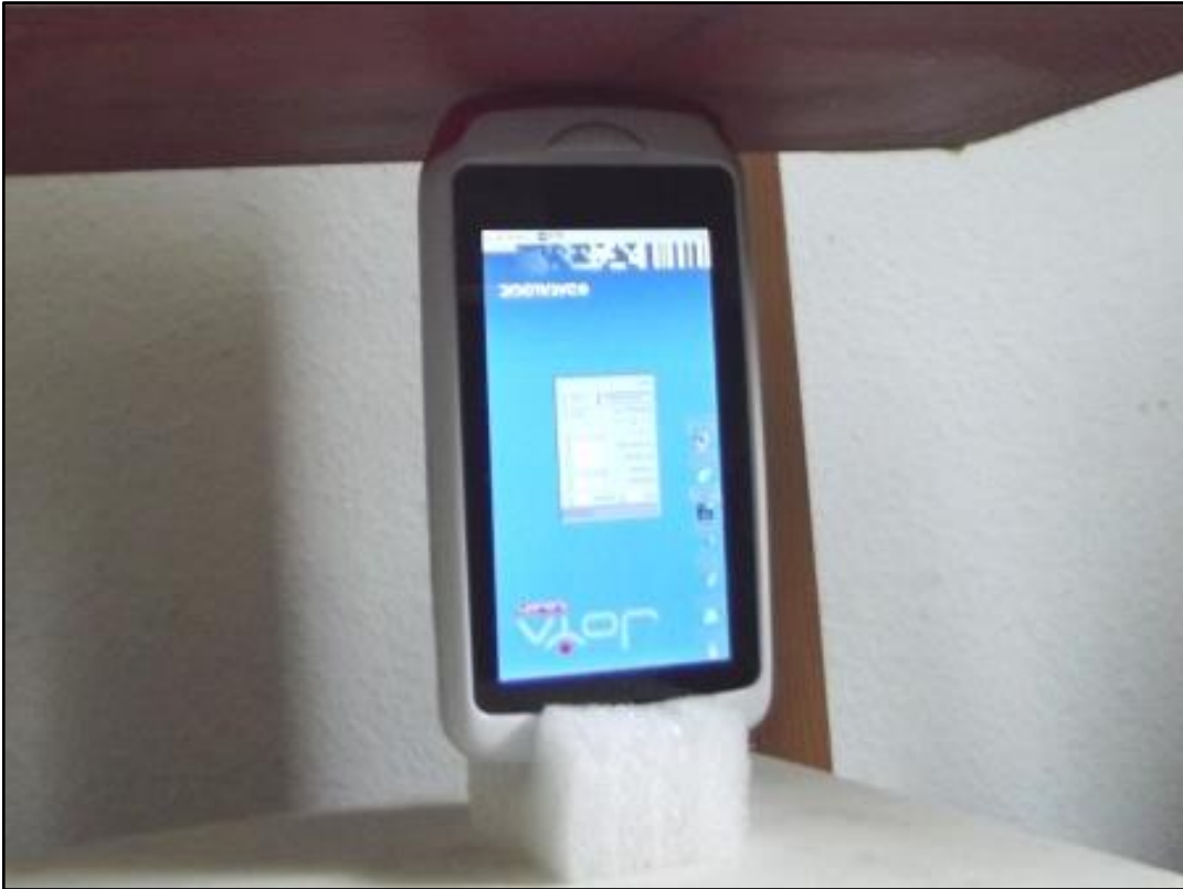
Photo 15: Test position bottom side with 0mm distance
