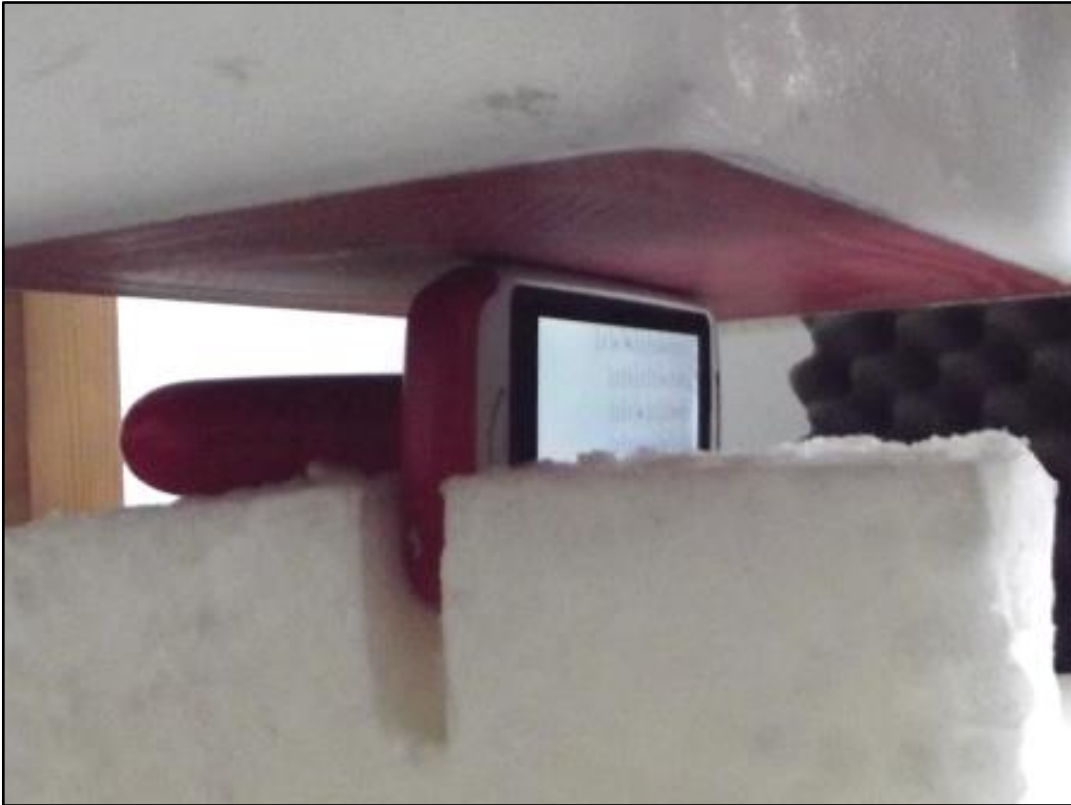
Photo 19: Test position left side with 0mm distance (Gun)
