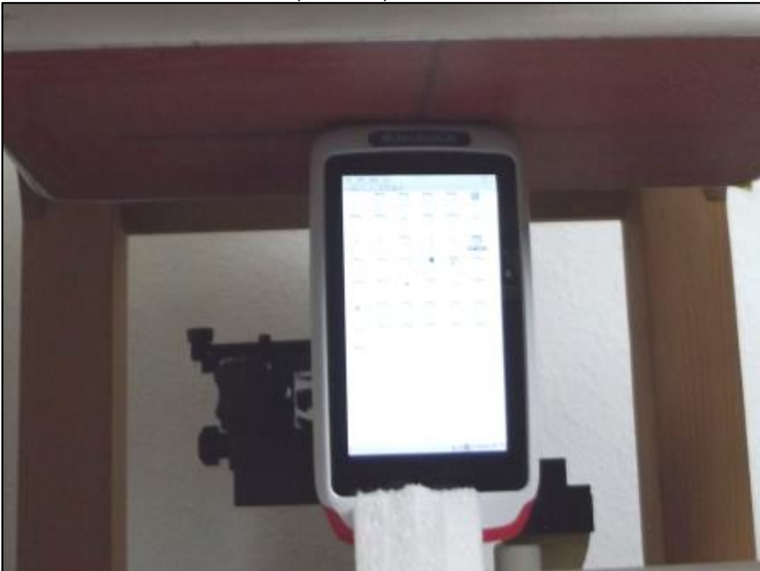
Photo 16: Test position top side with 0mm distance
