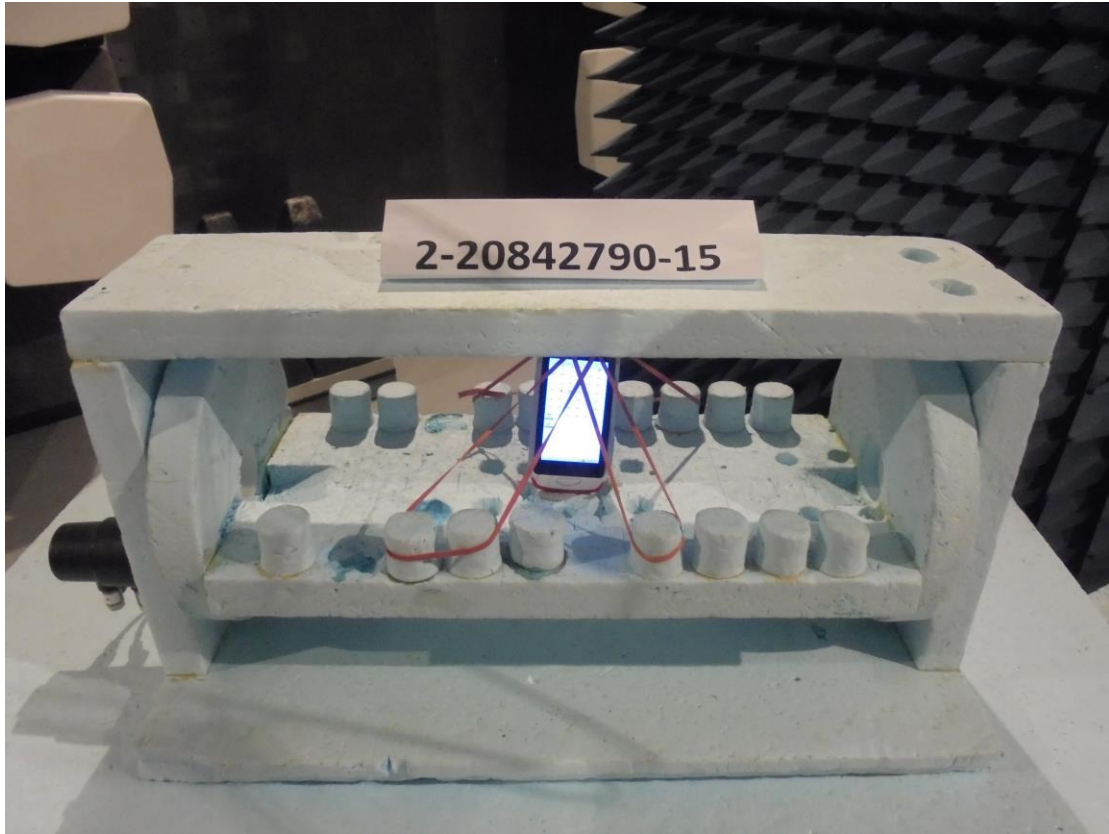
Photograph 8: Radiated measurement set-up (close up view_front side)_EUT 0°
