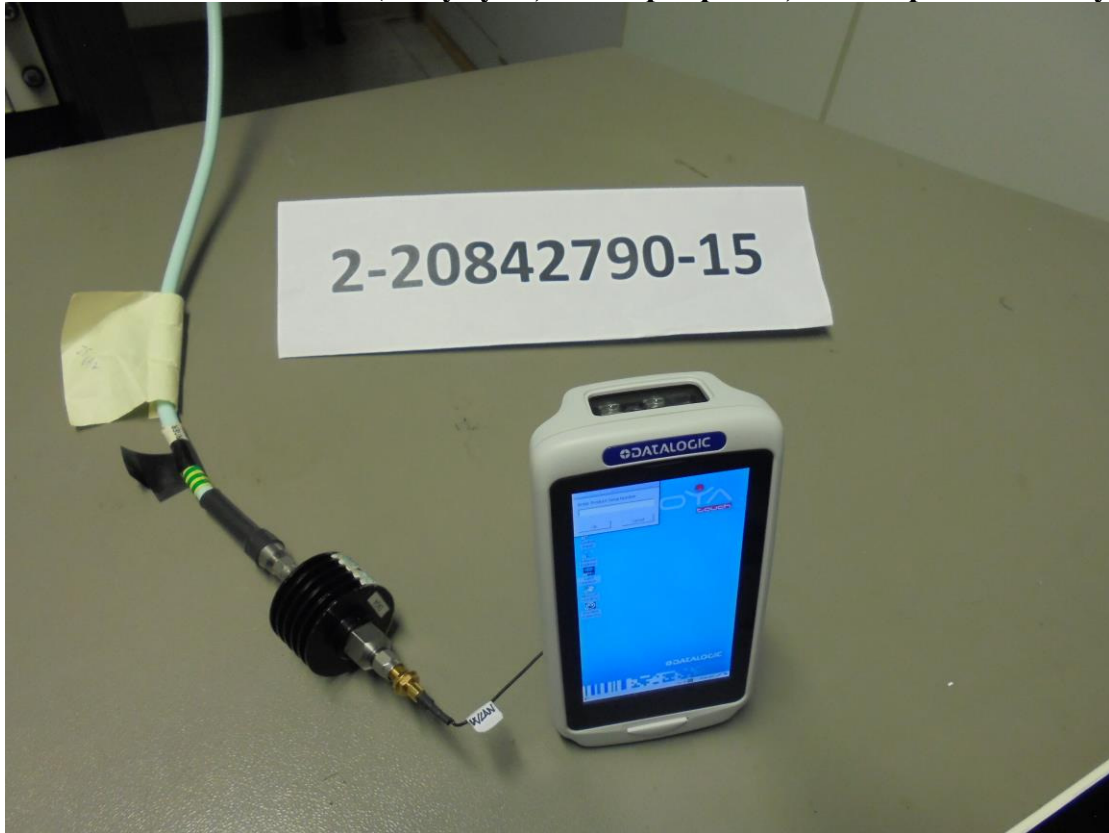
Photograph 1: Conducted measurement set-up (close up view_front side)
