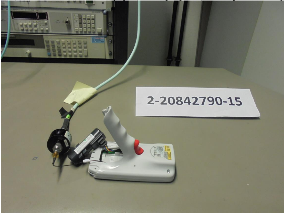
Photograph 1: Conducted measurement set-up (close up view_front side)
