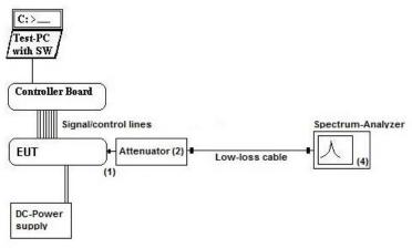
ANSI C63.10:2013, KDB 558074 D01 DTS Meas.Guidance v03r05 **Testing method:**
