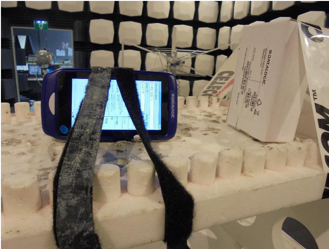
Photograph 8: Radiated measurement set-up (close up view_front side)_EUT 0°
