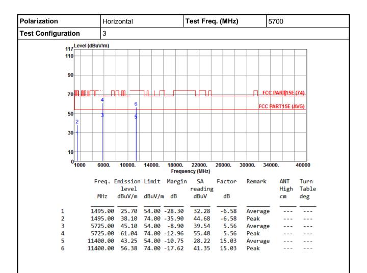
Note 1: ">20dB" means spurious emission levels that exceed the level of 20 dB below the applicable limit. Note 2: For restricted bands, the peak measurement is fully sufficient, as the max field strength as measured with the Peak-Detector meets the AV-Limit so that the AV level does not need to be reported in addition.
