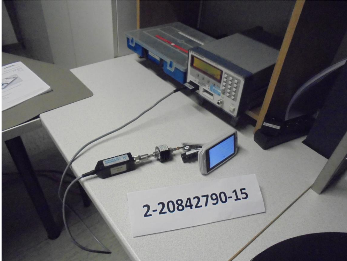
Photograph 3: Conducted measurement power meter set-up (overview_front side)
