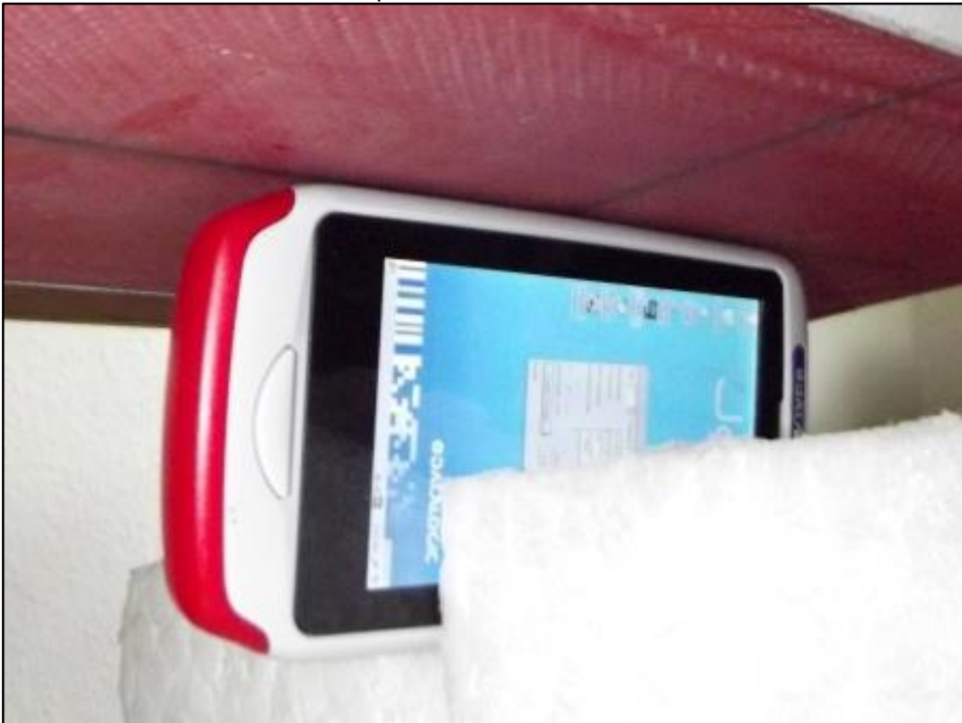
Photo 14: Test position left side with 0mm distance
