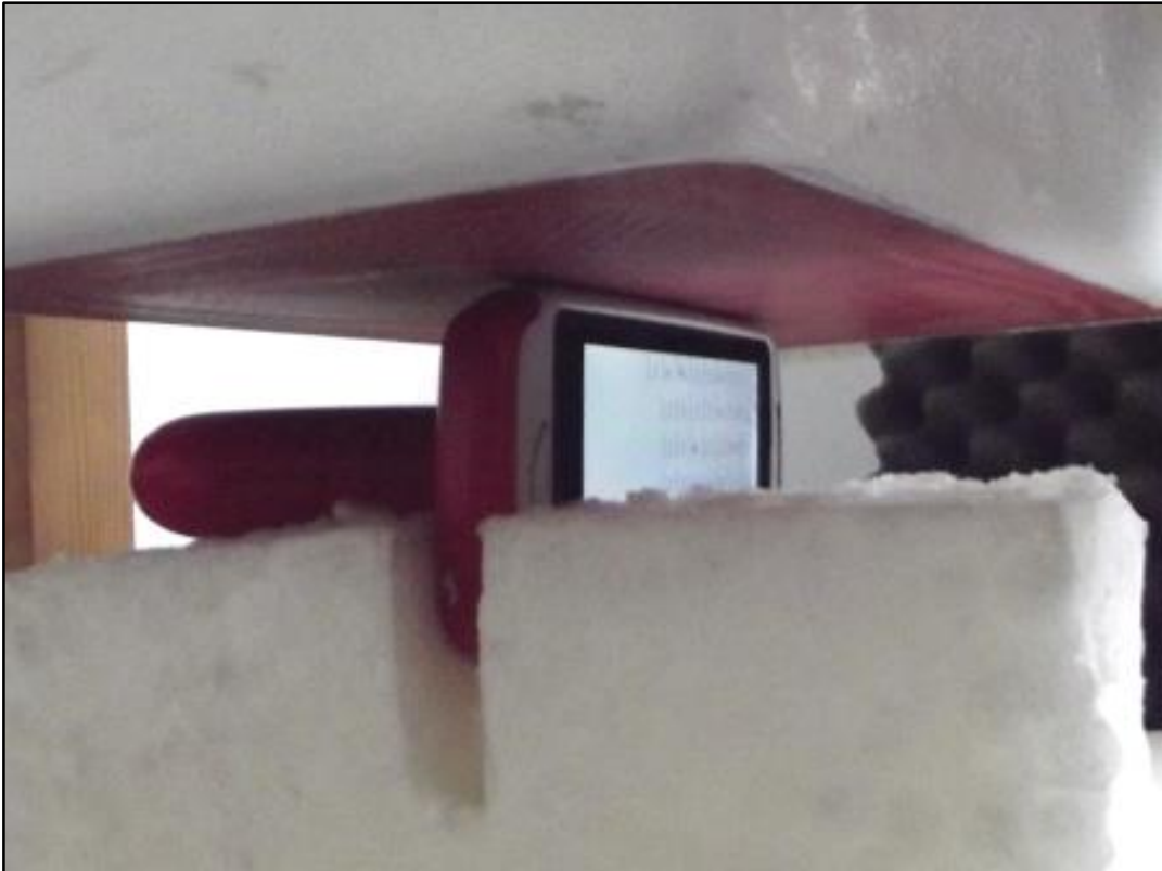
Photo 18: Test position left side with 0mm distance (Gun)
