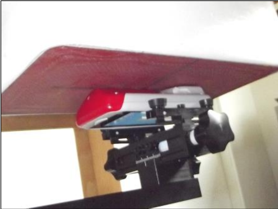
Photo 13: Test position rear side with 0mm distance
