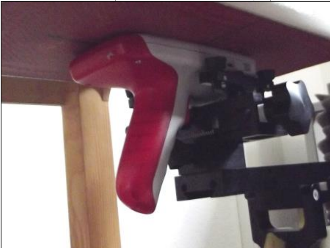
Photo 16: Test position front side with 0mm distance (Gun)
