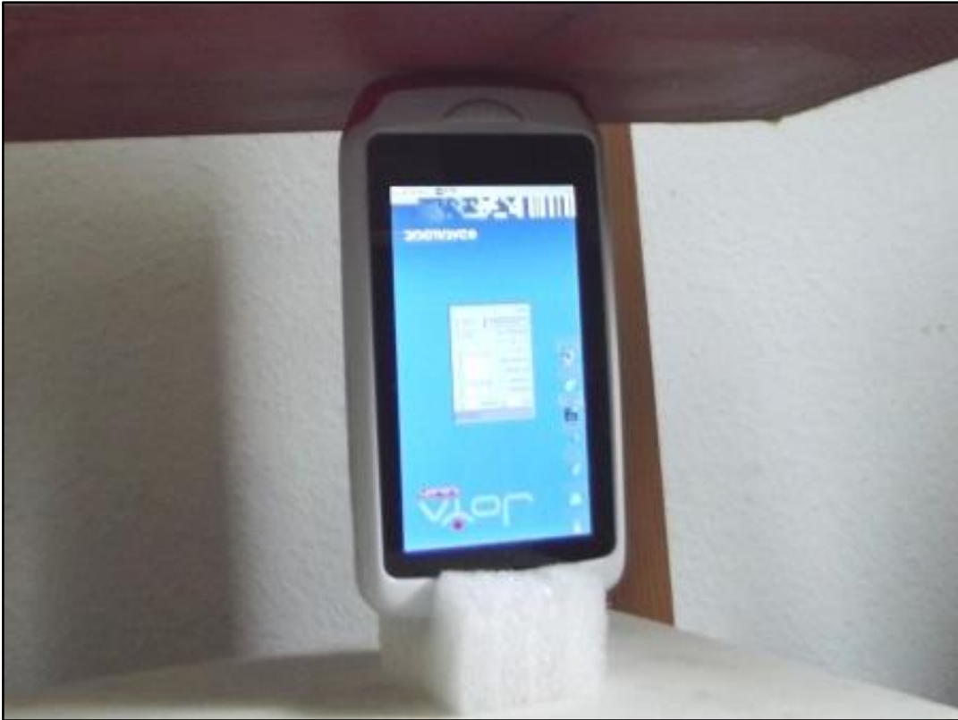
Photo 15: Test position bottom side with 0mm distance
