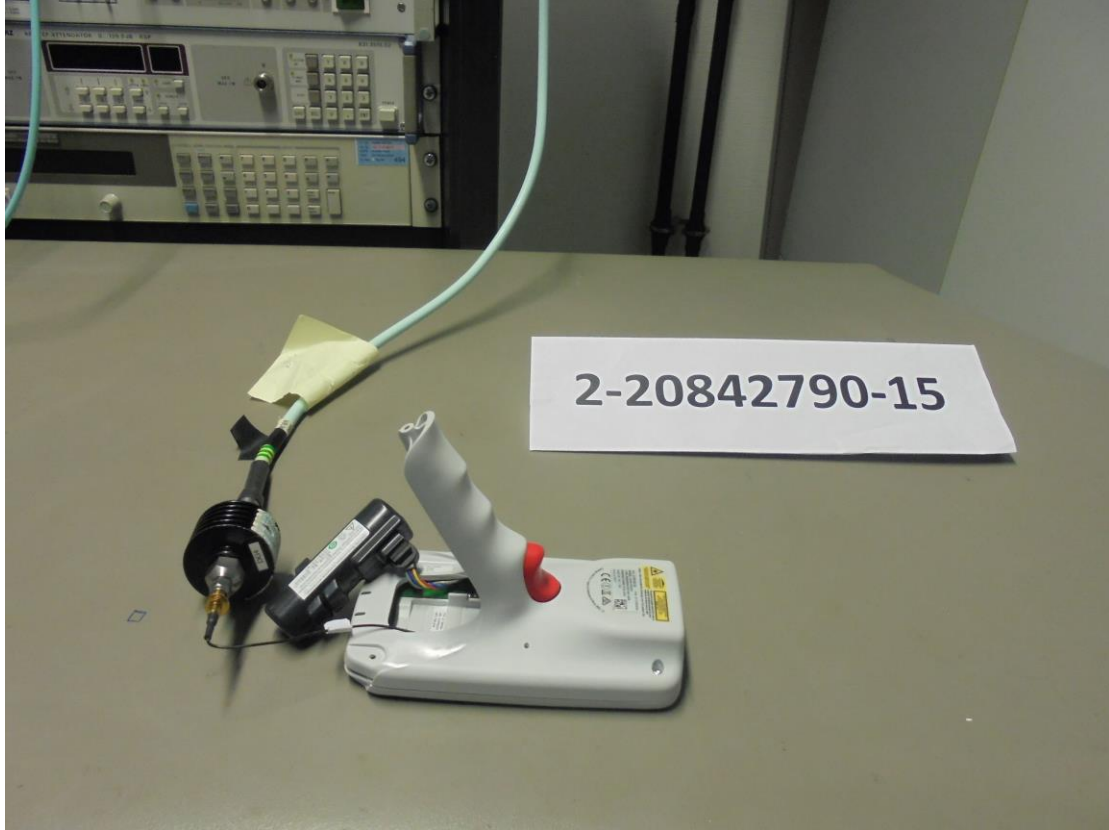
Photograph 1: Conducted measurement set-up (close up view_front side)
