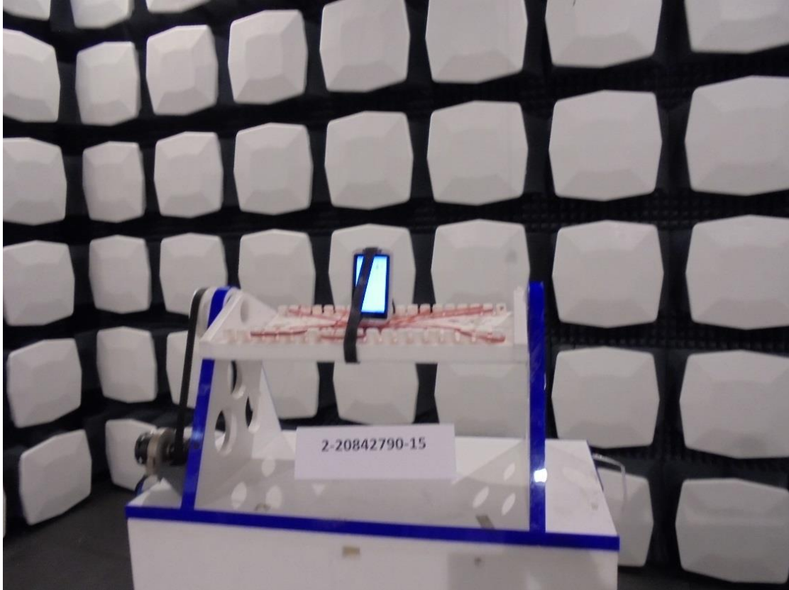
Photograph 14: Radiated measurement set-up (close up view_front side)_ EUT 0°
