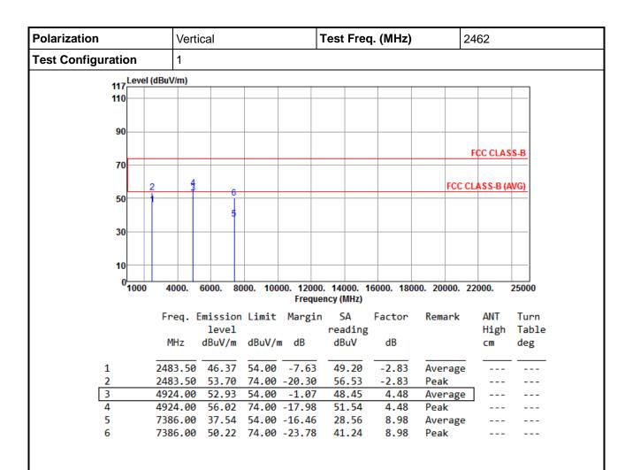
Note 2: For restricted bands, the peak measurement is fully sufficient, as the max field strength as measured with the Peak-Detector meets the AV-Limit so that the AV level does not need to be reported in addition.
