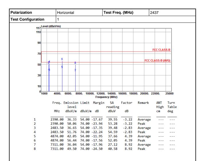
Note 2: For restricted bands, the peak measurement is fully sufficient, as the max field strength as measured with the Peak-Detector meets the AV-Limit so that the AV level does not need to be reported in addition.
