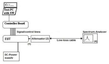
**Testing method:** ANSI C63.10:2013, KDB 558074 D01 DTS Meas.Guidance v03r05
