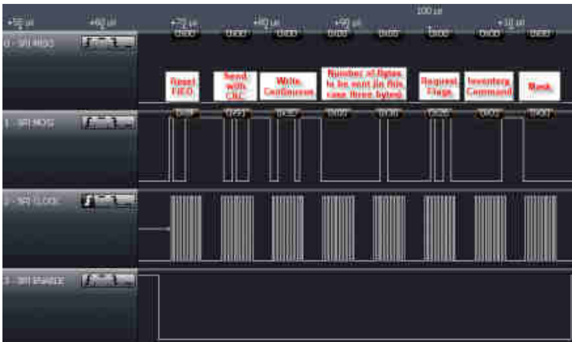
Figure 6-22. Inventory Command Sent From MCU to TRF7970A
