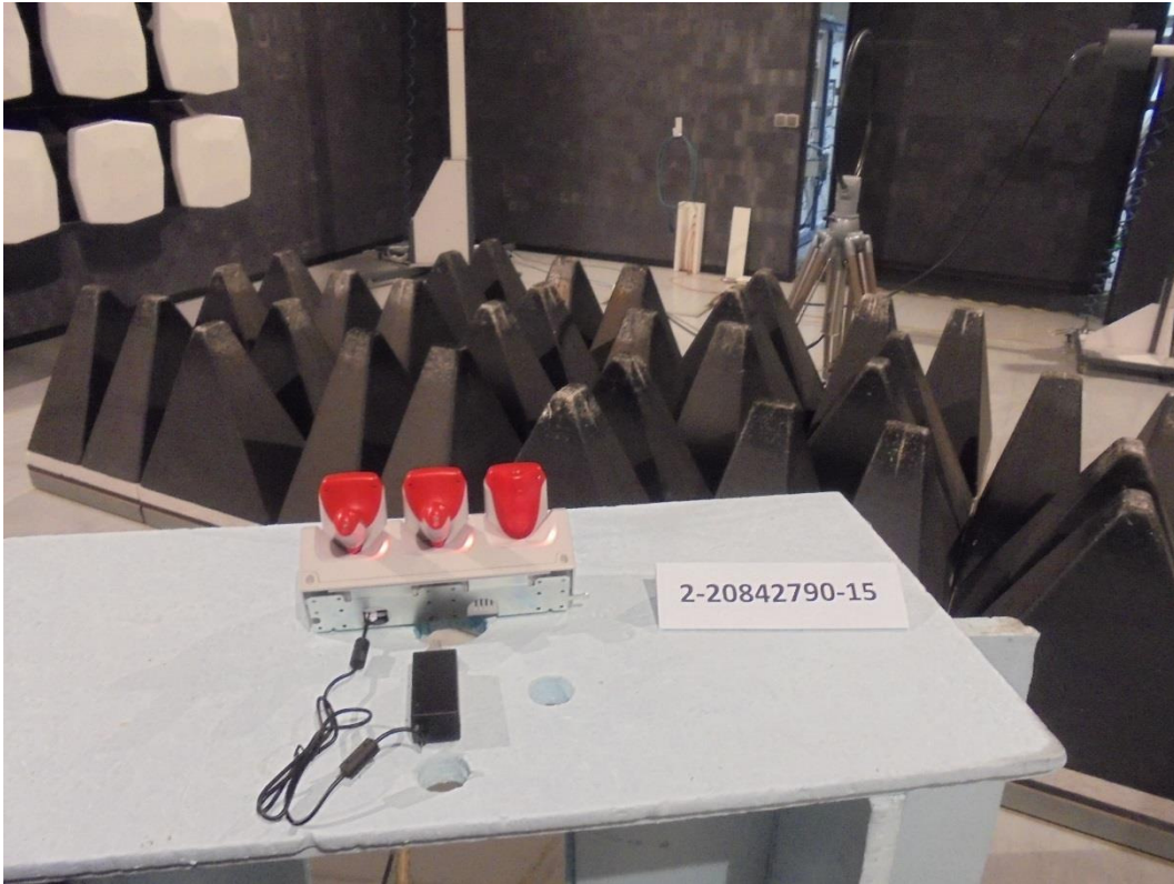
Photograph 3: Radiated measurement set-up (close up view_ back side)
