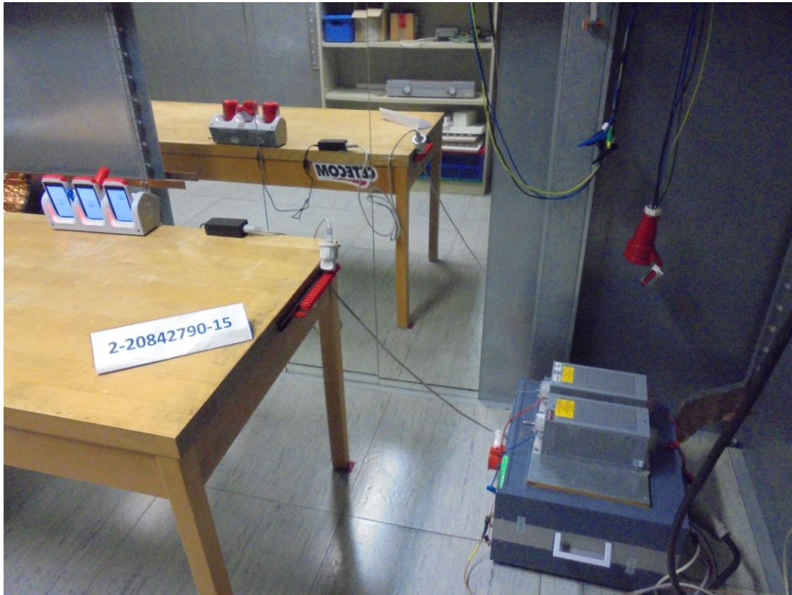
Photograph 9: AC Power Lines Conducted Emissions set-up (overview_front side)
