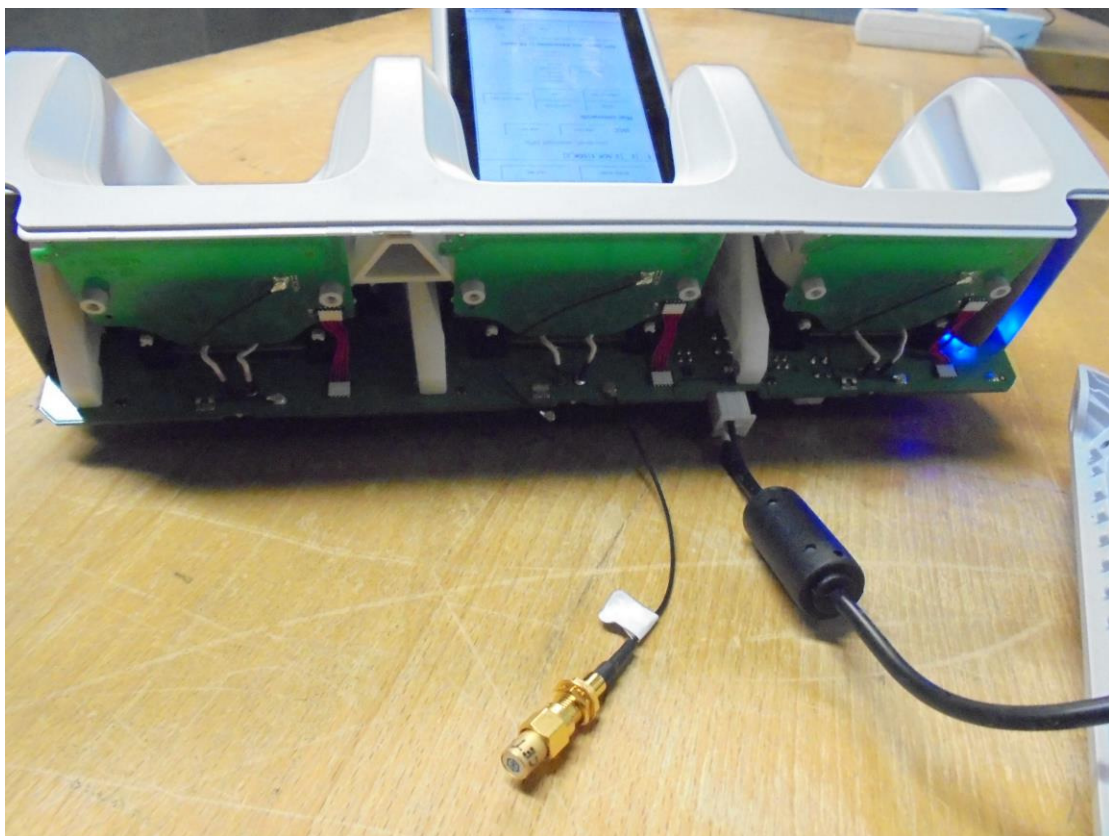
Photograph 12: AC Power Lines Conducted Emissions set-up (NFC Output 50 Ohm Termination)
