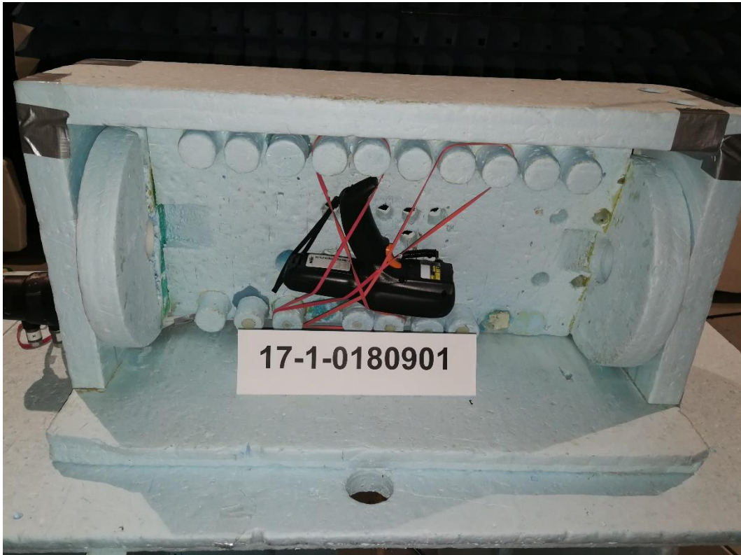
Photograph 5: Set Up 1-Close View -9 kHz-30 MHz- EUT Laying 90°- Front Side
