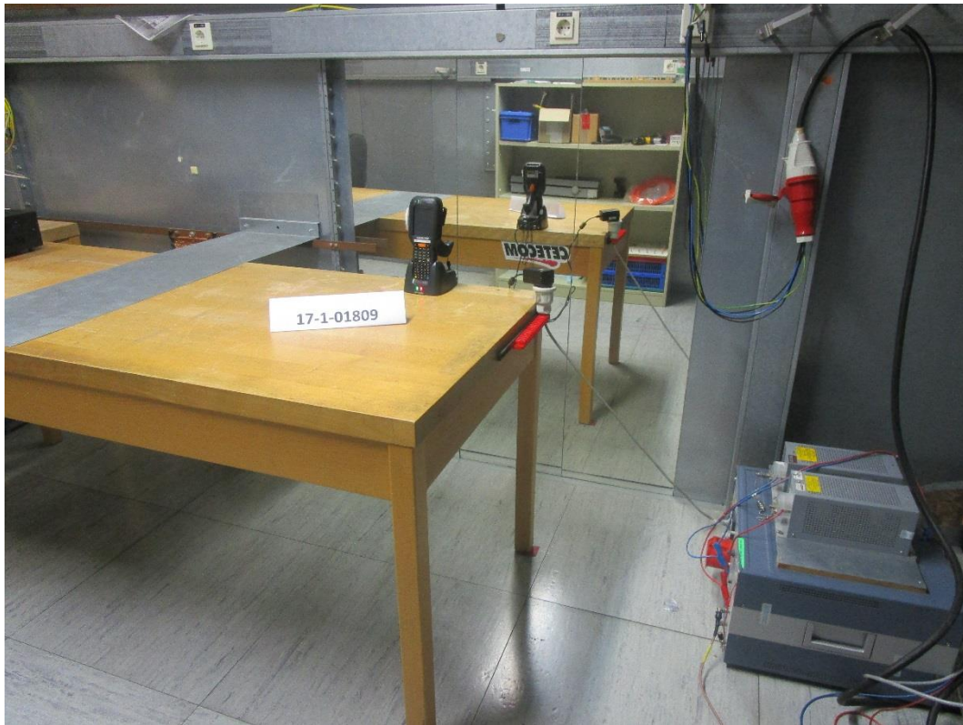
Photograph 1: Set Up 1-Overall View- Terminal & Spare Battery Charging via Docking Station
