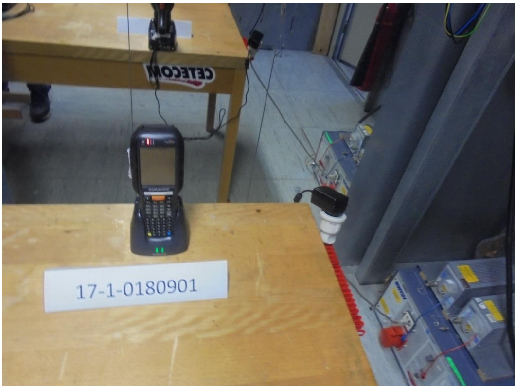
Photograph 2: Set Up 1-Close View- Terminal & Spare Battery Charging via Docking Station
