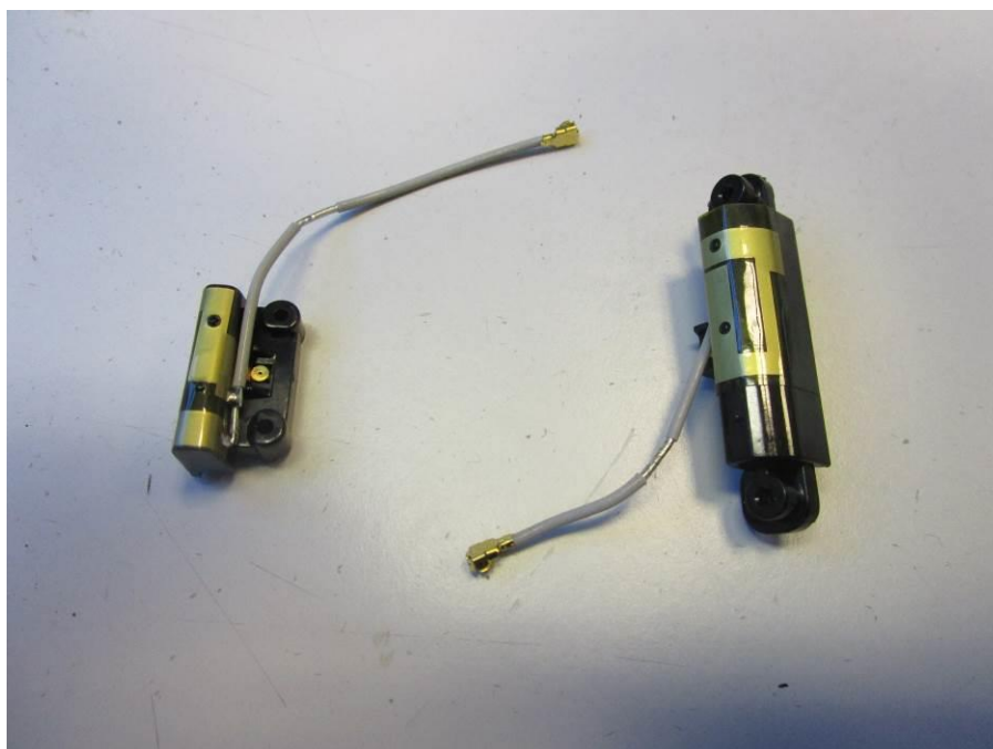
Photograph 23: FALCON X4 –Integrated Antennas ANT2 (on left) & ANT1 (on right)
