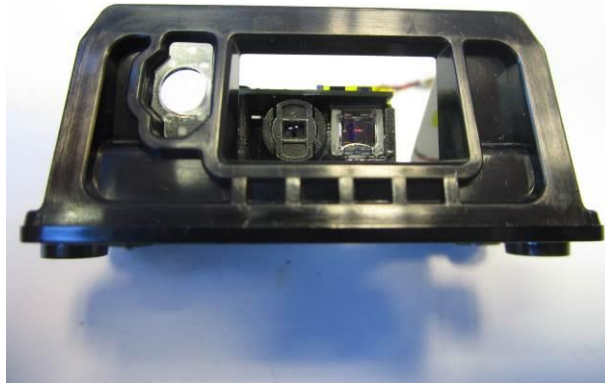
Photograph 16: FALCON X4 – Barcode Reader Assembly-1D Imager
