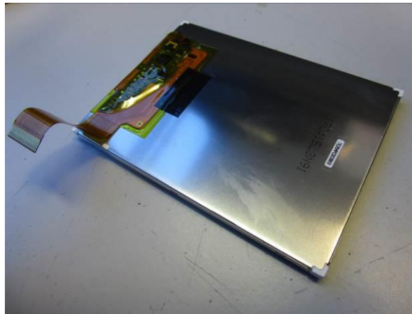
Photograph 9: FALCON X4 –Display Assembly Back Side
