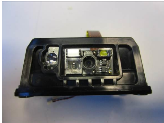
Photograph 17: FALCON X4 – Barcode Reader Assembly-2D Imager
