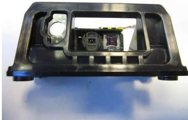
Photograph 18: FALCON X4 – Barcode Reader Assembly-1D Imager
