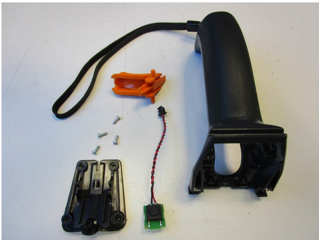
Photograph 4: FALCON X4 – Handle Assembly disconnected
