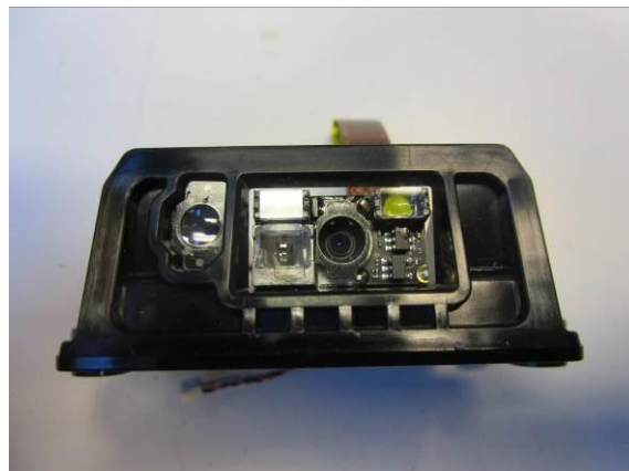
Photograph 19: FALCON X4 – Barcode Reader Assembly-2D Imager
