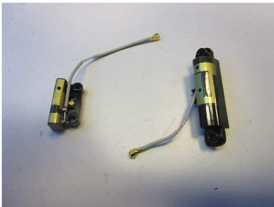
Photograph 25: FALCON X4 –Integrated Antennas ANT2 (on left) & ANT1 (on right)
