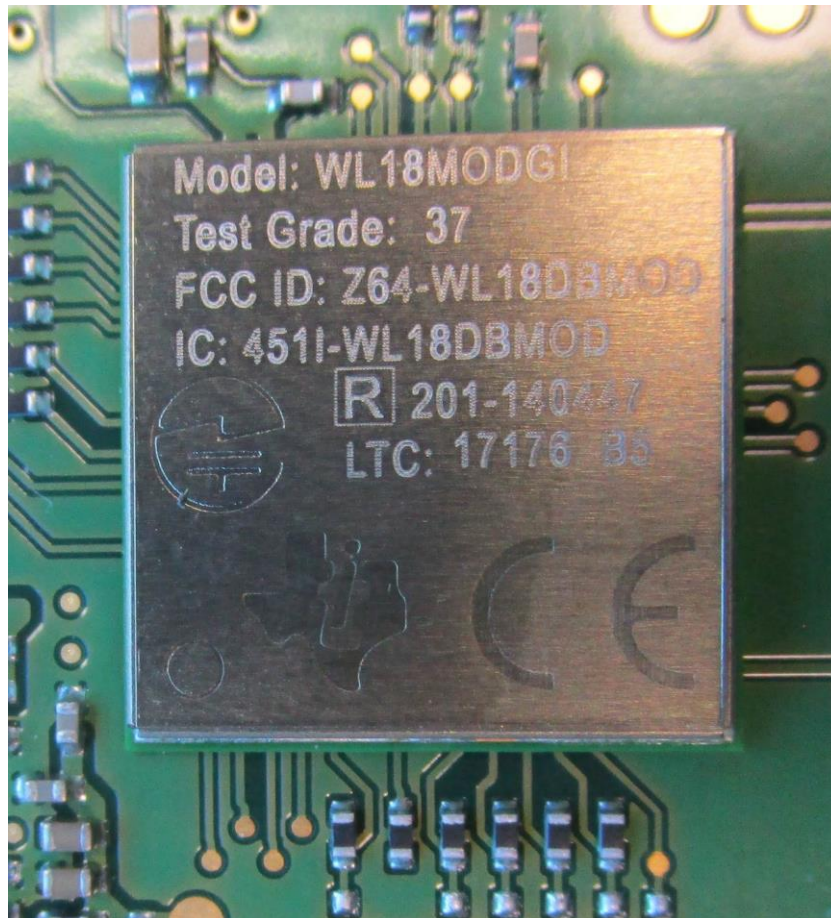
Photograph 24: FALCON X4 –Integrated Radio Module- WL18MODGI
