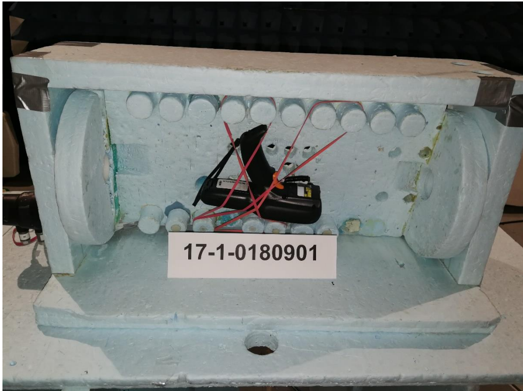
Photograph 7: Set Up 1-Close View -9 kHz-30 MHz- EUT Laying 90°- Front Side
