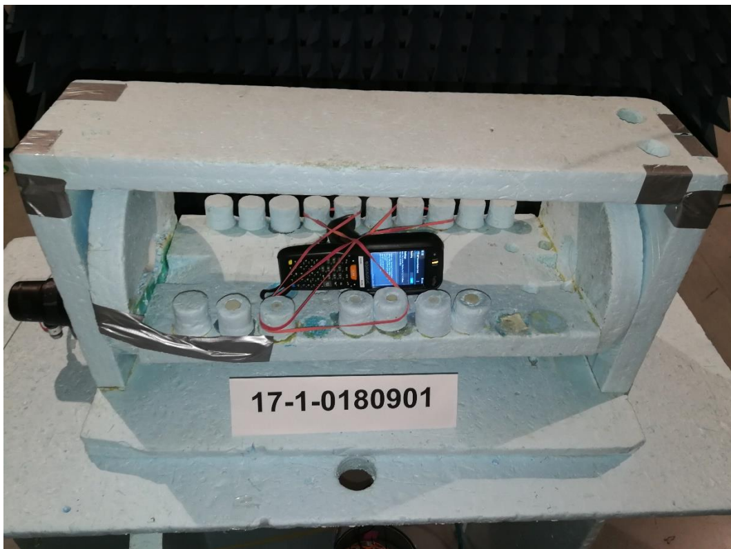
Photograph 8: Set Up 1-Close View -9 kHz-30 MHz- EUT Laying 0°- Front Side
