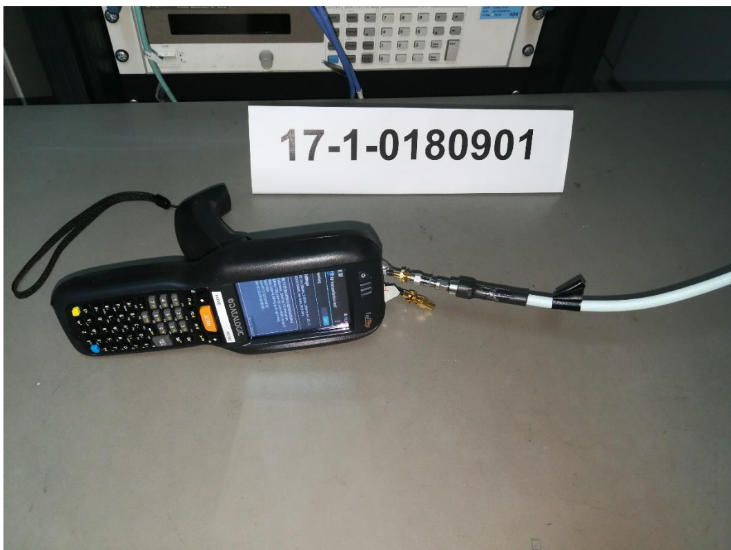
Photograph 4: Set Up 2-Close View-ANT1 Used + ANT2 Terminated with 50 \Omega
