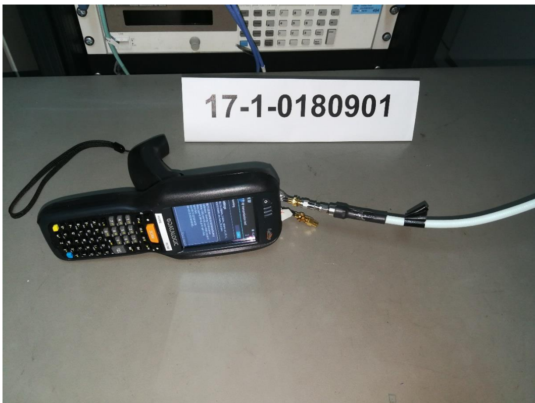
Photograph 6: Set Up 2-Close View- ANT1 Used + ANT2 Terminated with 50 \Omega
