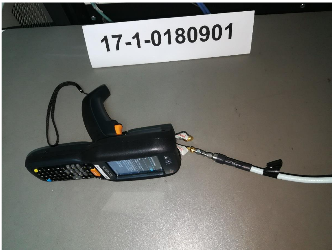
Photograph 8: Set Up 2-Close View- ANT2 Used + ANT1 Terminated with 50 \Omega
