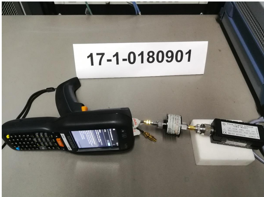
Photograph 2: Set Up 2-Close View-ANT1 Used + ANT2 Terminated with 50 \Omega
