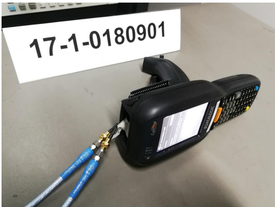
Photograph 10: Set Up 2-Close View- ANT2 + ANT1 used [WLAN n Mode-MIMO]
