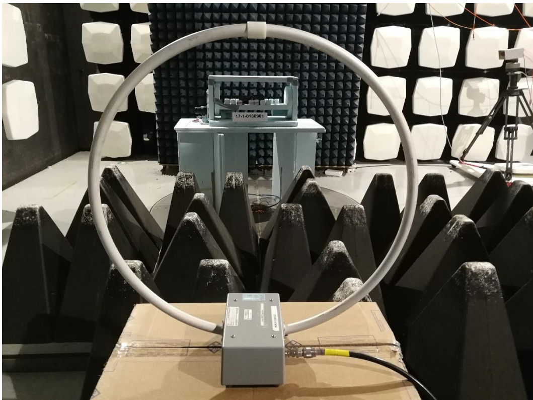
Photograph 12: Set Up 1-Overall View- 9 kHz-30 MHz- EUT Laying 0° - Front Side
