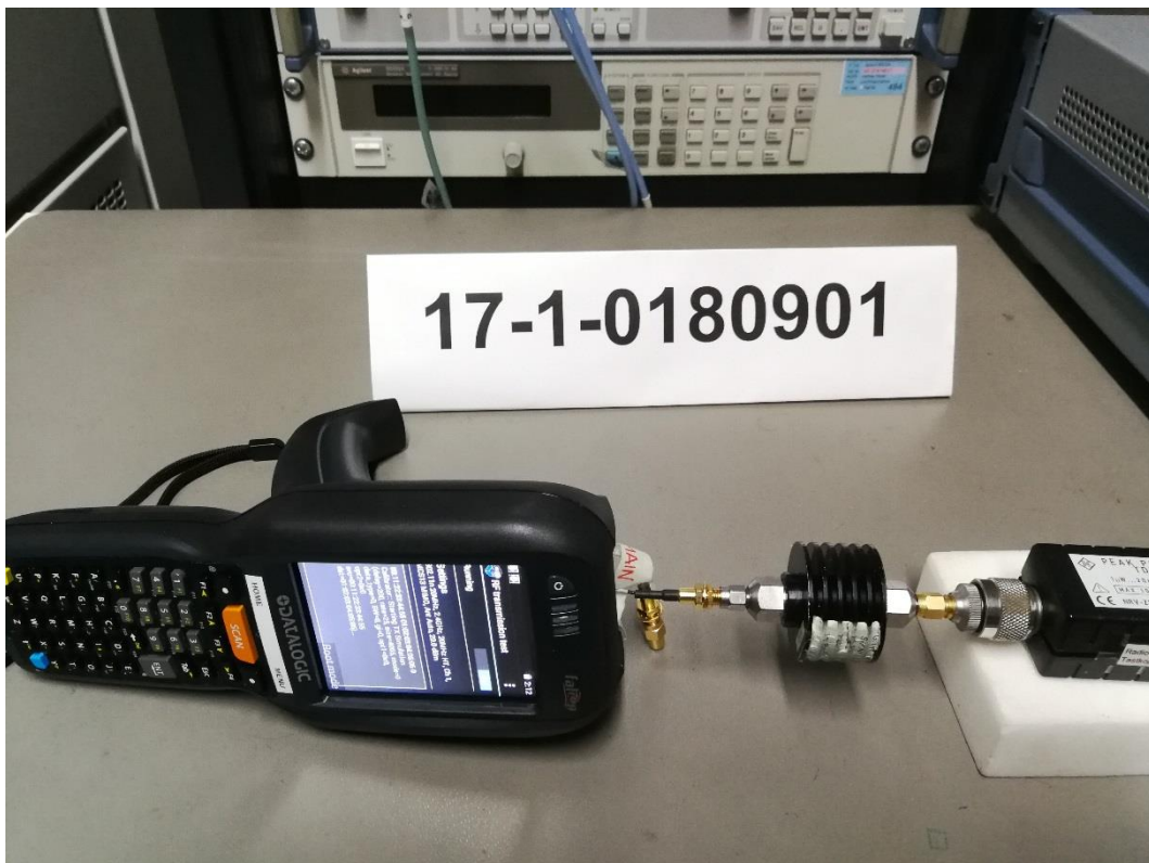
Photograph 4: Set Up 2-Close View-ANT2 Used + ANT1 Terminated with 50 \Omega
