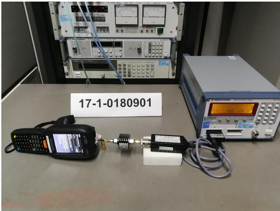
Photograph 3: Set Up 2-Overall View-ANT2 Used + ANT1 Terminated with 50 \Omega
