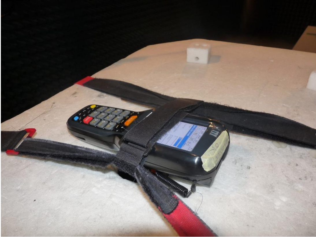
Photo 1: Test setup for FCC 15.247 and FCC 15.407
