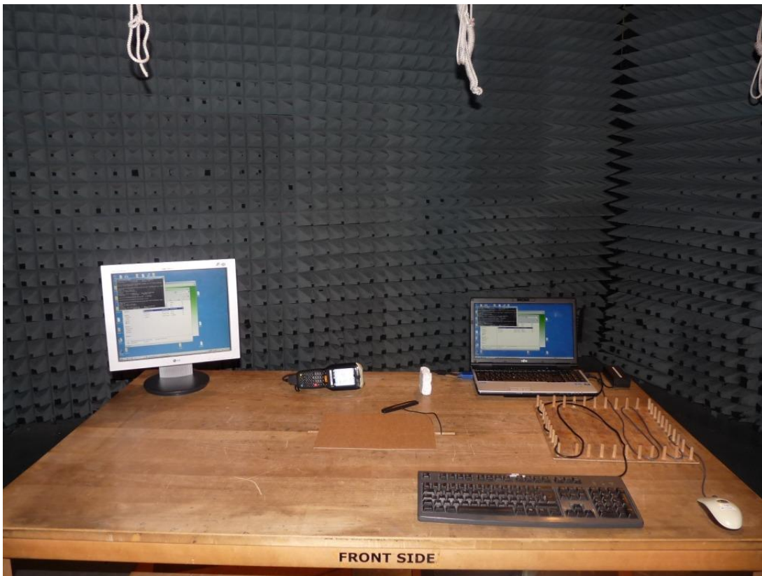
Photo 1: Test setup for radiated measurements (unintentional radiator §15)
