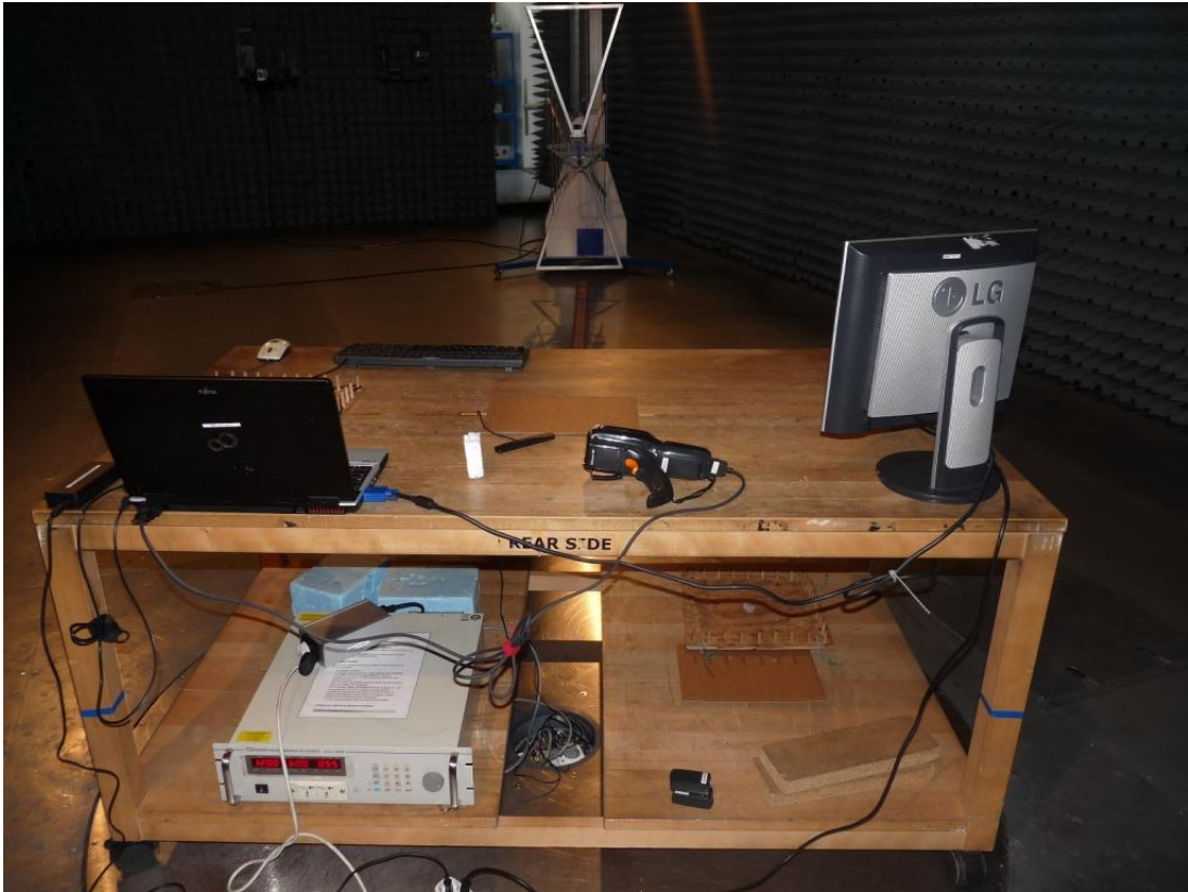
Photo 2: Test setup for radiated measurements (unintentional radiator §15)
