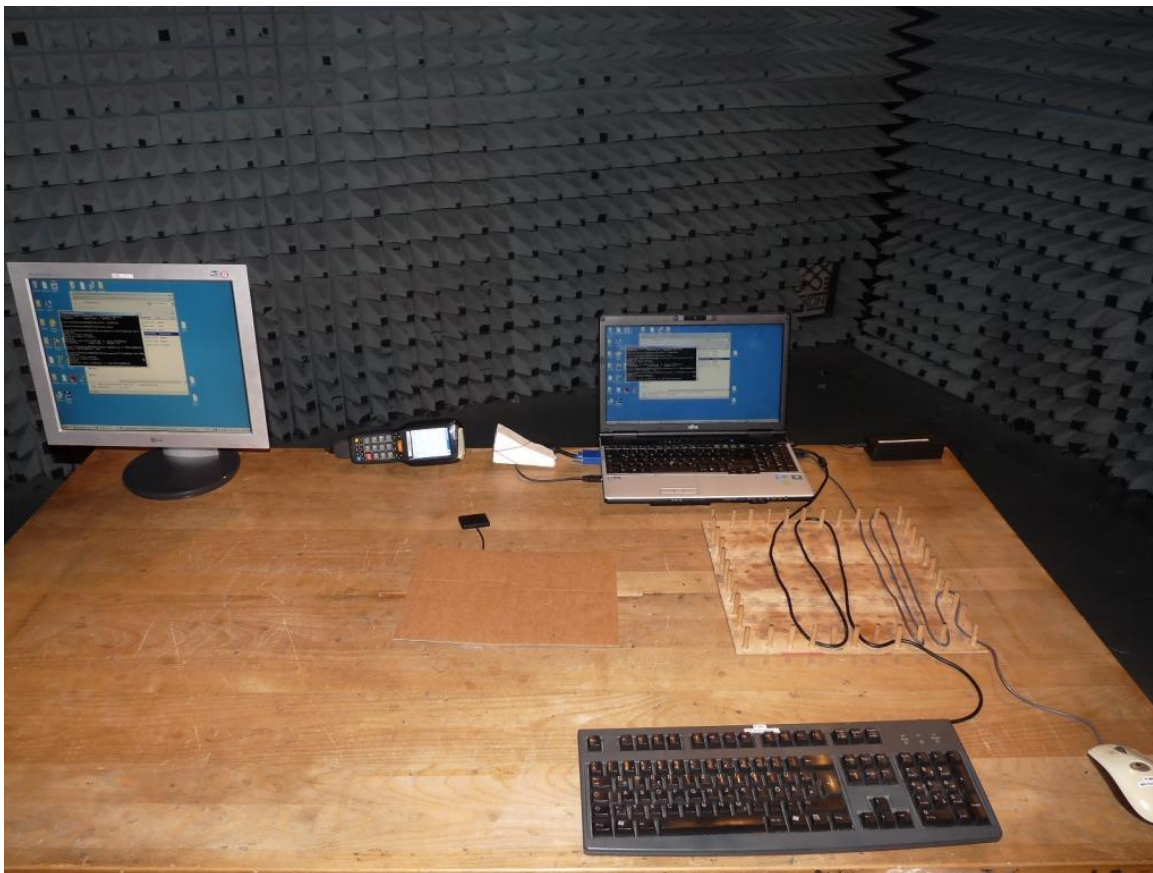
Photo 3: Test setup for radiated measurements (unintentional radiator §15), front view, Setup AA01
