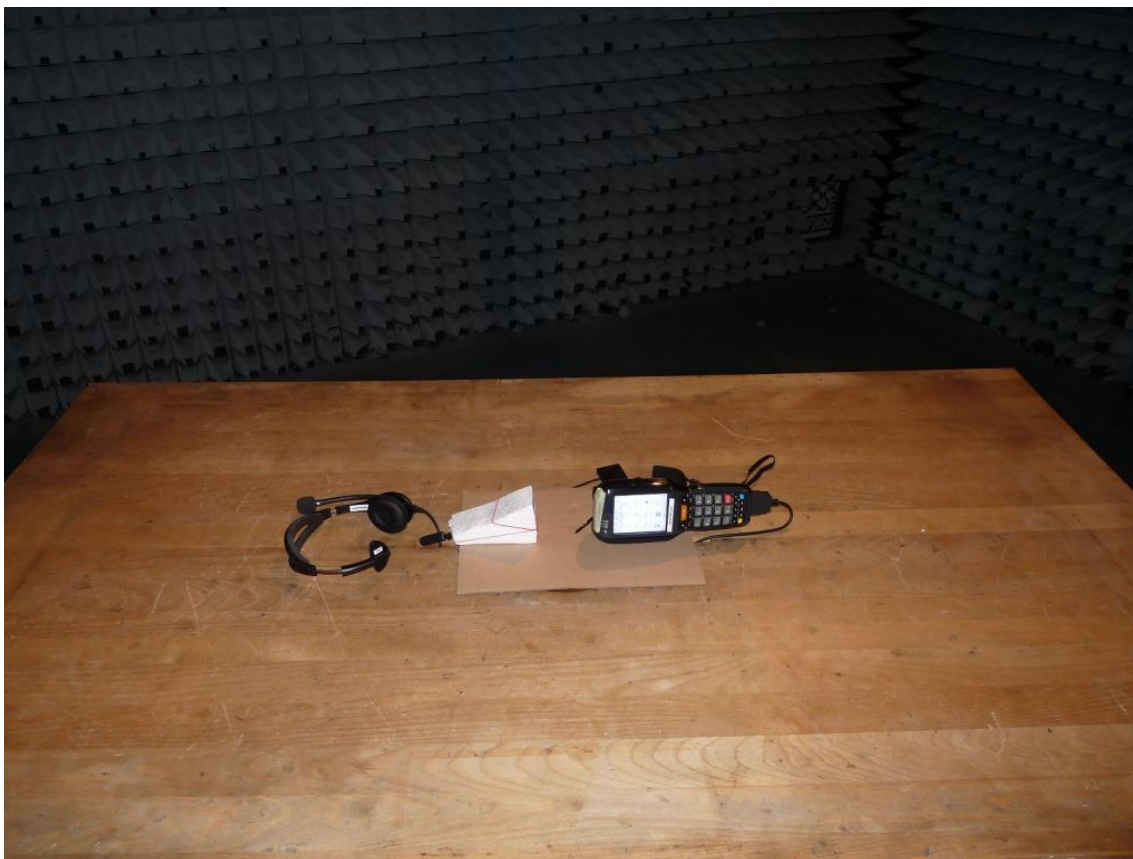
Photo 5: Test setup for radiated measurements (unintentional radiator §15), front view, Setup AB01
