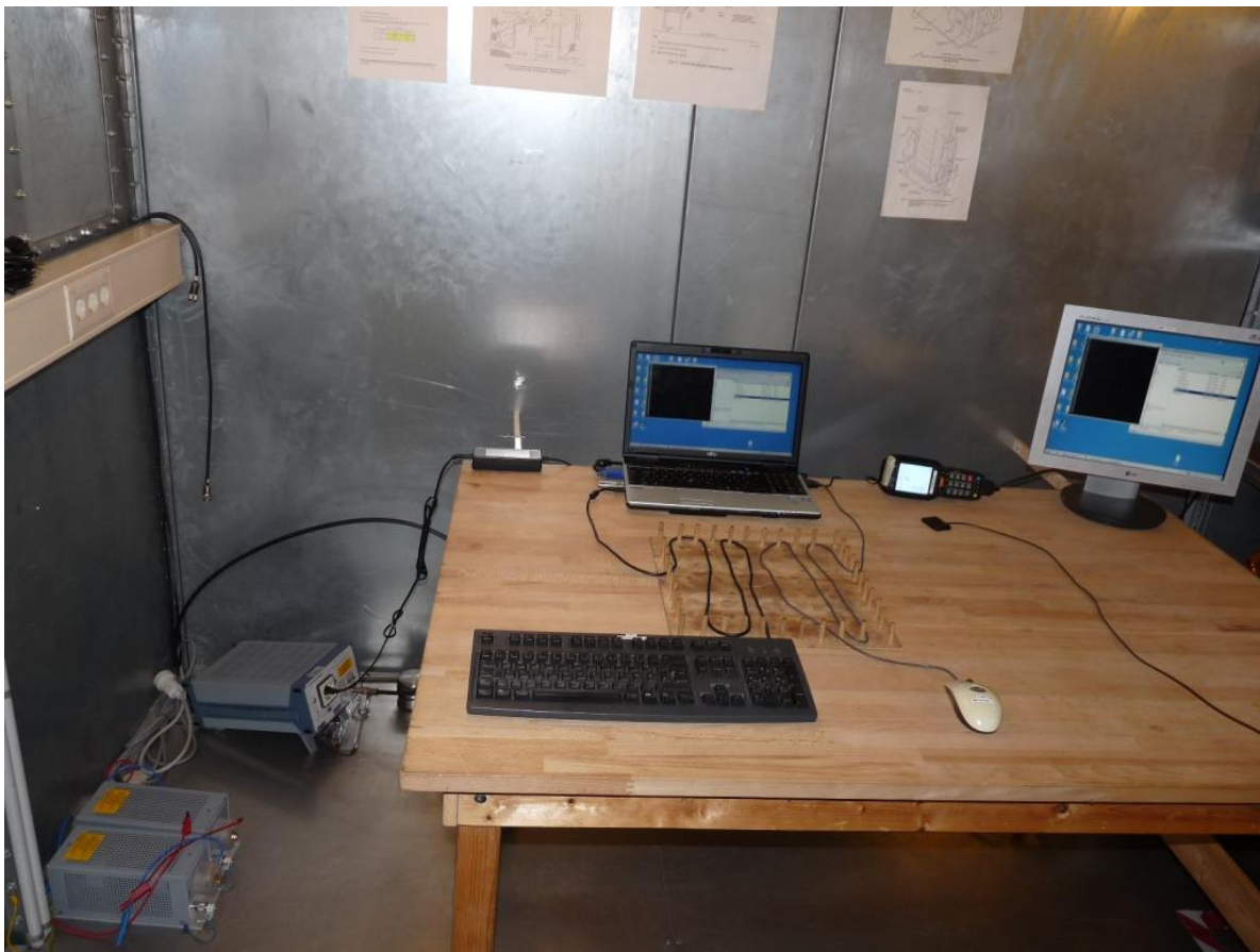
Photo 1: Test setup for conducted measurements (AC Port (power line), unintentional radiator §15), Setup AA01
