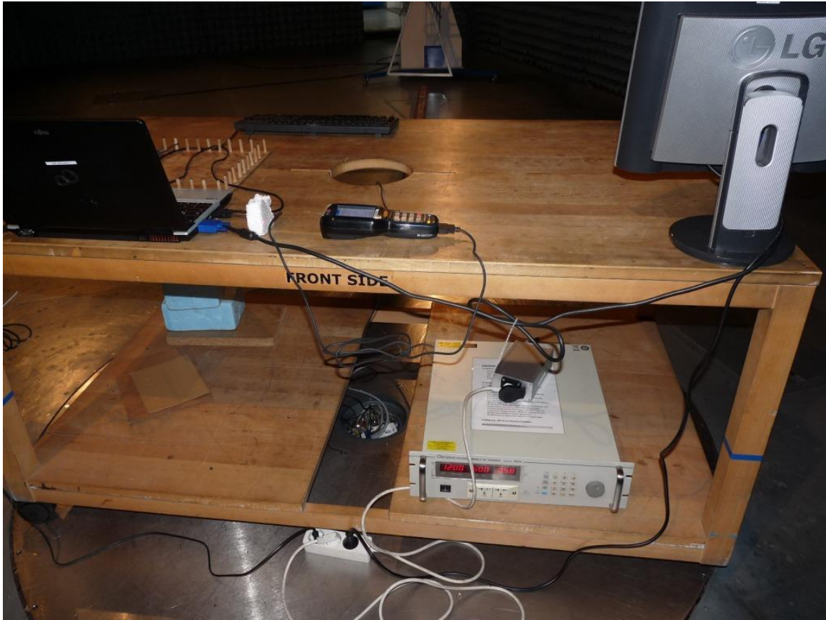
Photo 8: Test setup for radiated measurements (unintentional radiator §15), rear view, Setup AF01
