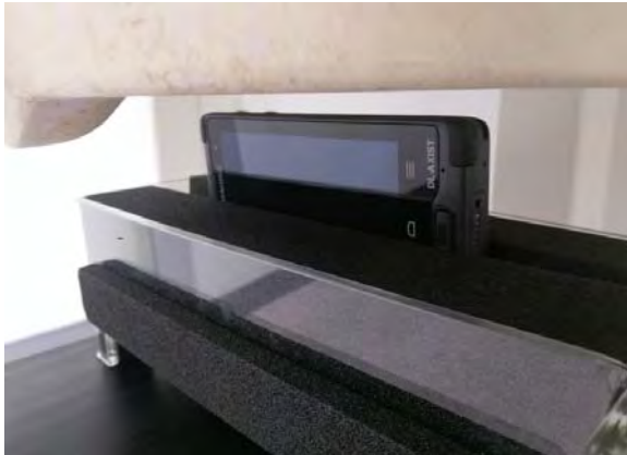
Fig.13 EUT Right side to flat phantom
