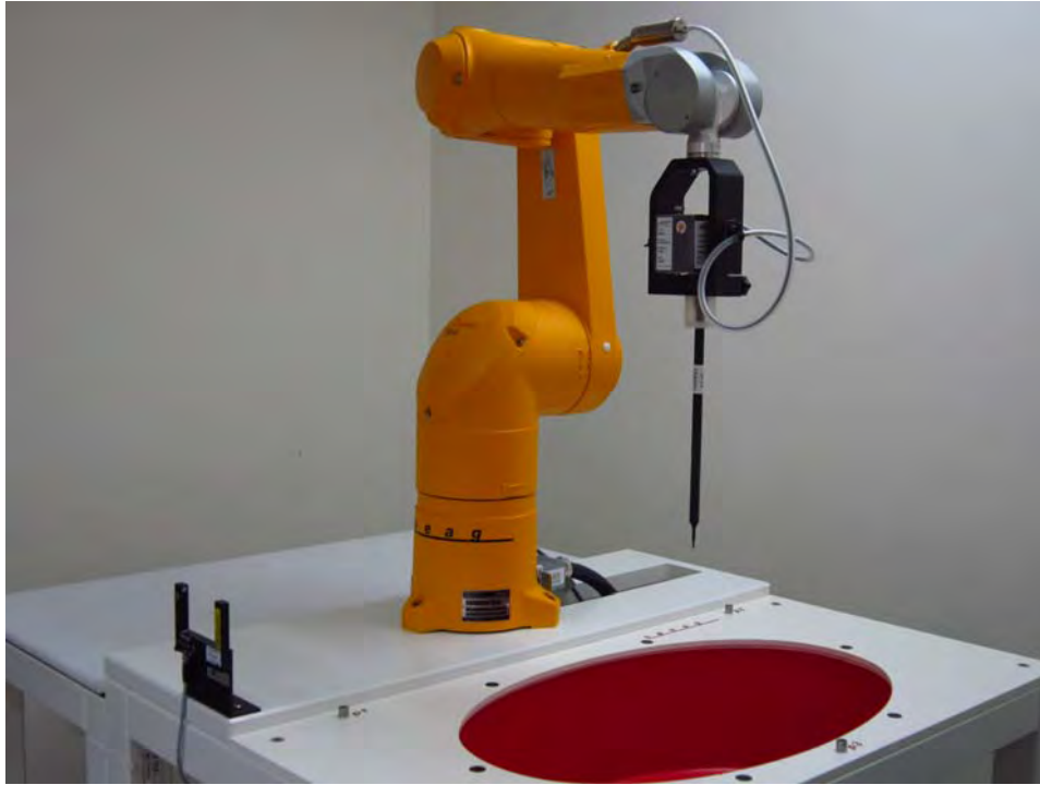
Fig.1 Photograph of the SAR measurement system
