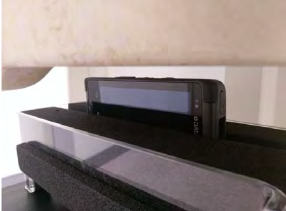
Fig.12 EUT Left side to flat phantom
