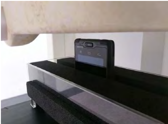
Fig.10 EUT Bottom side to flat phantom
