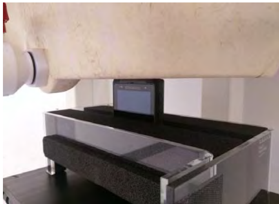
Fig.17 EUT Top side to flat phantom
