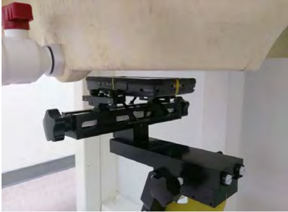
Fig.9 EUT Front side to flat phantom
