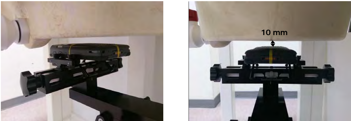
Fig.8 EUT Back side to flat phantom
