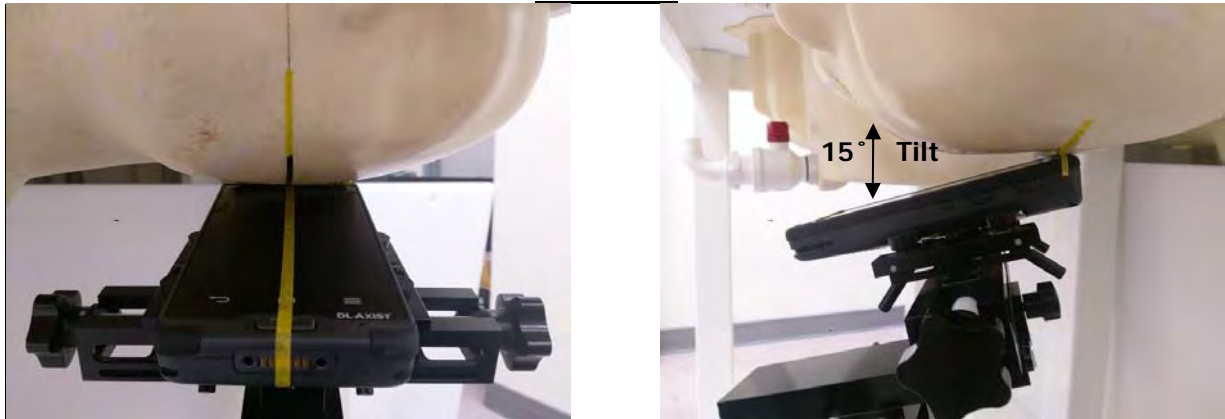
Fig.6 Left Head Section / Ear-Tilt Position(15°)
