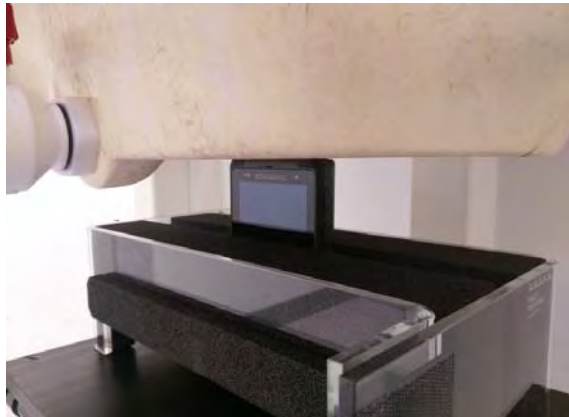
Fig.17 EUT Top side to flat phantom
