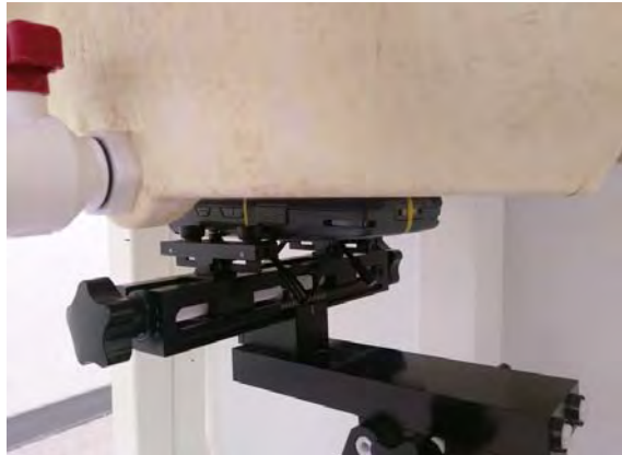
Fig.16 EUT Front side to flat phantom
