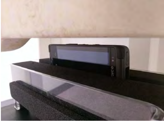
Fig.12 EUT Left side to flat phantom
