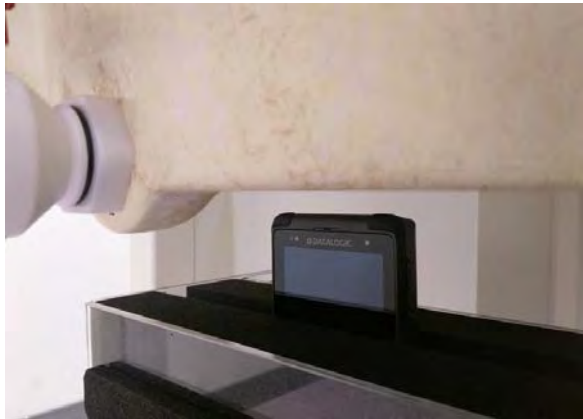
Fig.14 EUT Top side to flat phantom
