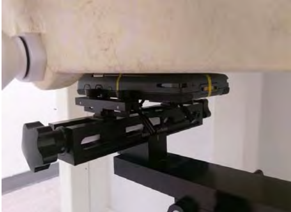
Fig.15 EUT Back side to flat phantom
