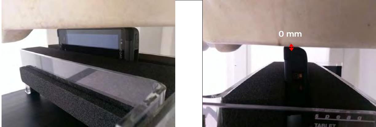
Fig.18 EUT Left side to flat phantom
