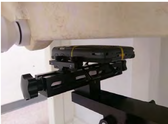
Fig.11 EUT Back side to flat phantom
