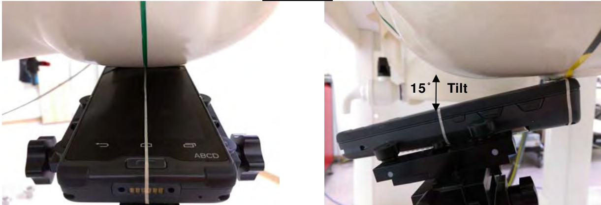
Fig.6 Left Head Section / Ear-Tilt Position(15°)
