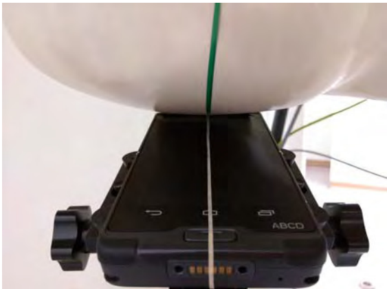
Fig.4 Right Head Section / Ear-Tilt Position(15°)
