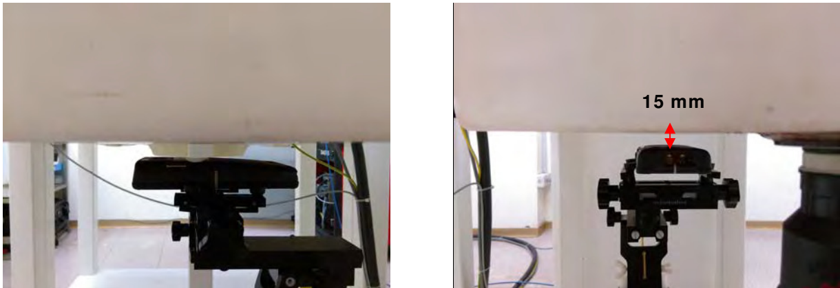
Fig.8 EUT Back to flat phantom
