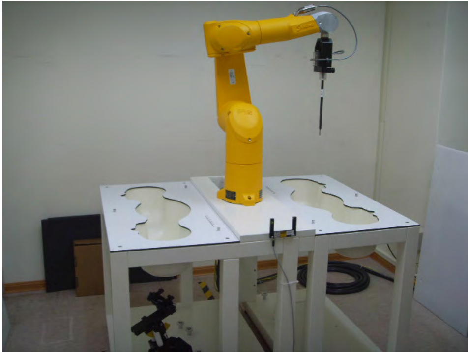
Fig.1 Photograph of the SAR measurement system
